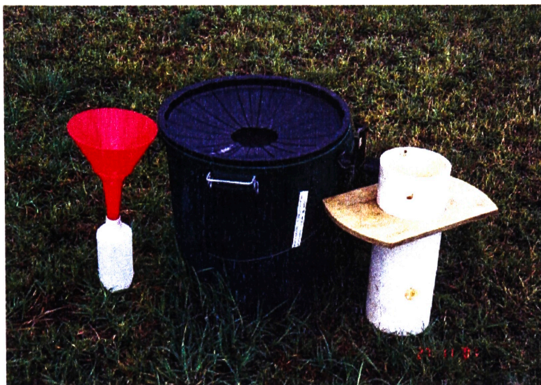
Figure 3.1: Cost effective rainfall sampling device.
