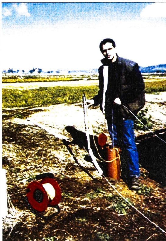
Figure 1: Hudson site A) View toward the top of the ridge from the lower slope (248110) B) Lithological profile exposed in the gully that crosses the mid-lower slope C) Groundwater piezometer and OTT automatic groundwater level logger at the Hudson agricultural trial site, displayed by S. Heidenreich.
