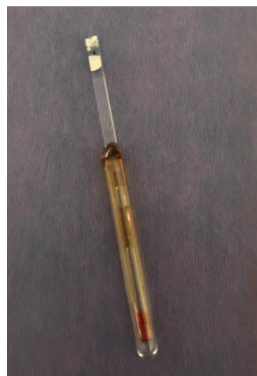
Figure 3.8: a) Photo of OLED device held by EDMR sample holder b) Photo of OLED device encapsulated inside an MD5 EPR tube.
