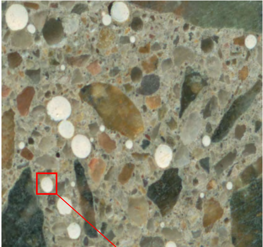
Figure 3.3.8 4800 ppi true optical resolution
