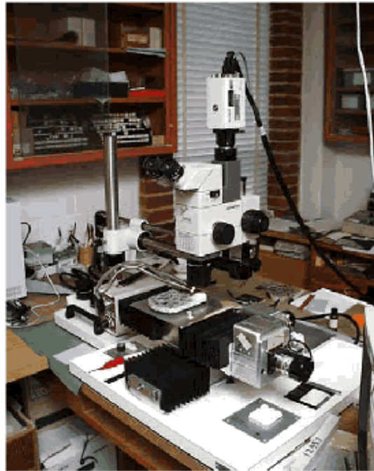
Figure 56. Partially automated linear traverse equipment for determining air-void parameters.
