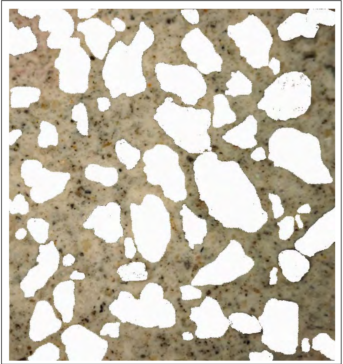
4 - Masked sand particles and porosity in white - Dar1
