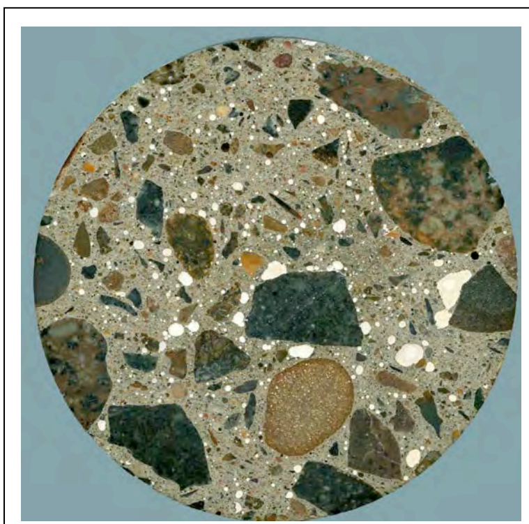
Figure 3.3.3.2.4 Fully filled Reference Sample 5b 4800 ppi, 48-24 bit colour, 1GB, 18856 x 18968 pixels (ready for a calculation in ImageJ)
