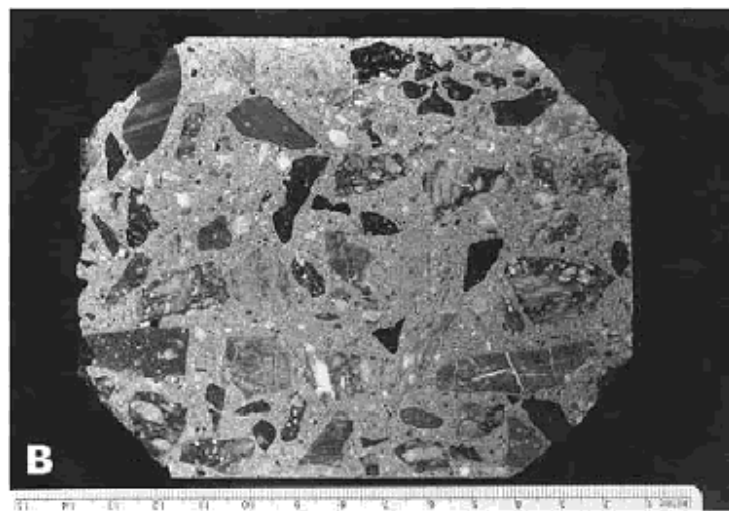
Figure 62. Finely lapped slices of concrete with normal paste content: Angular crushed granite coarse aggregate and fine sand aggregate.
