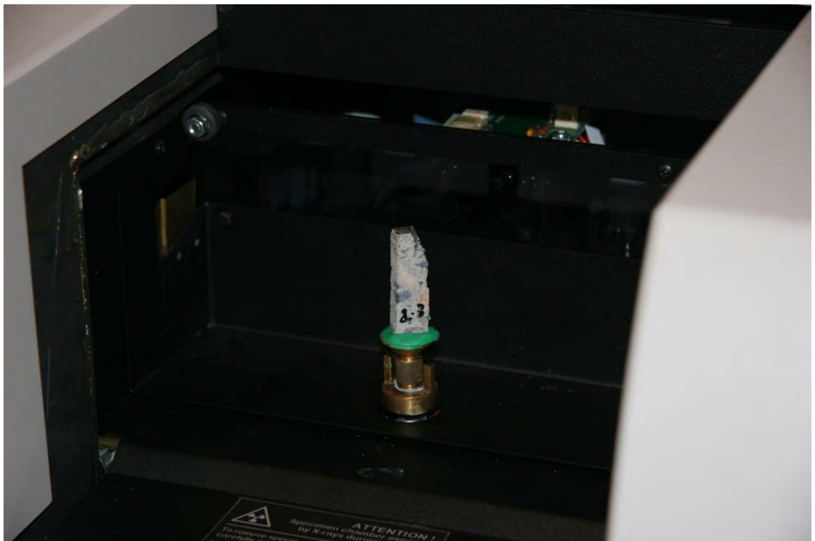
Figure 3.2.4 Close up of sample 2-3 loaded and held in static mode for 2D analysis
