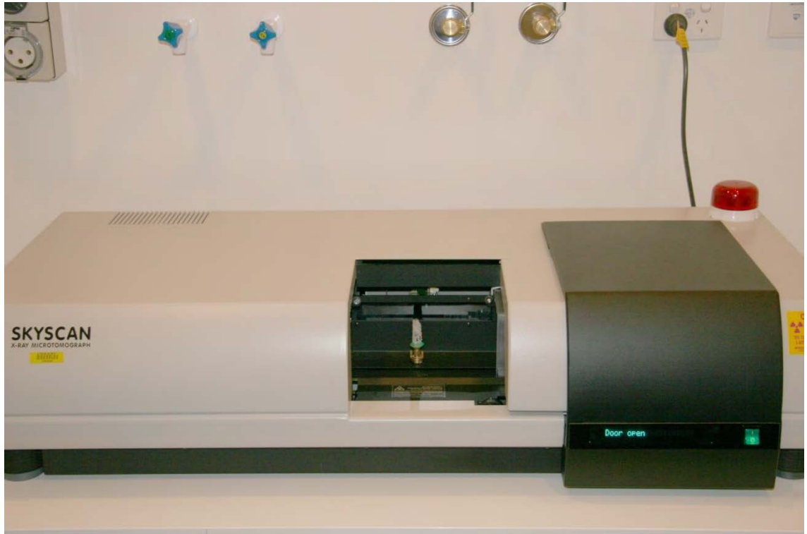
Figure 3.2.3 Skyscan X-Ray Microtomograph 1072 Micro CT (sample loaded)
