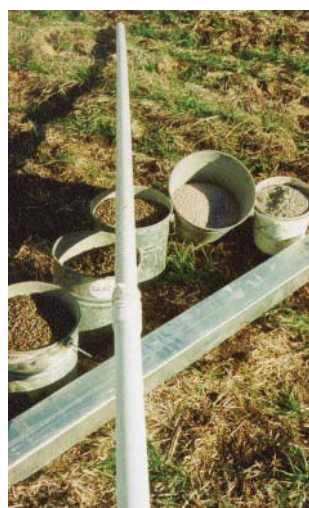
Figure 3 – Materials to install a shallow monitoring piezometer
