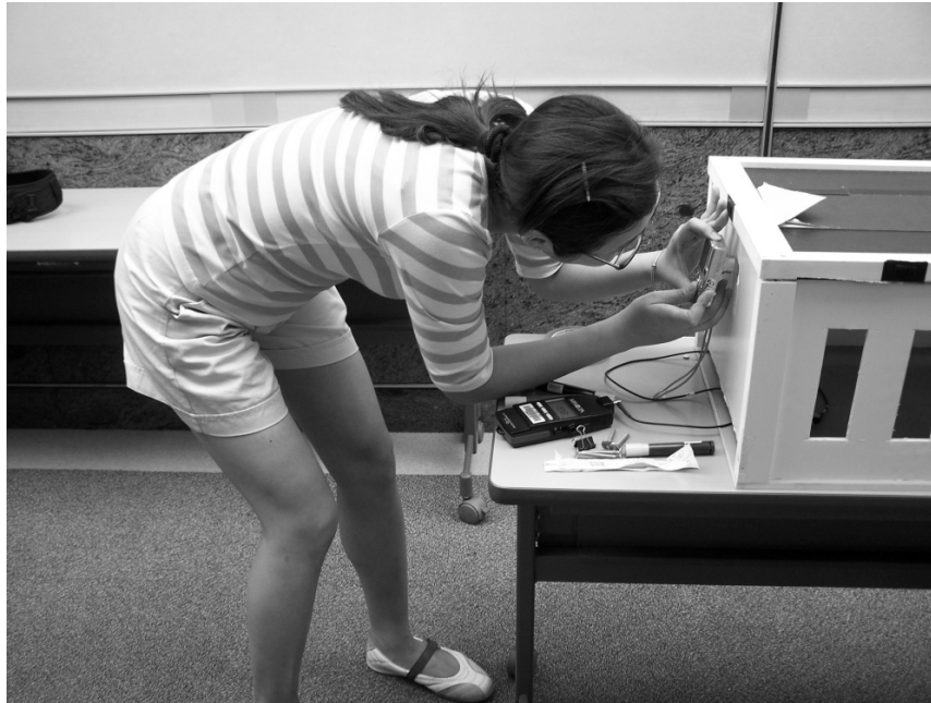
Figure 3: A student measuring the lighting levels and taking the photographs of a space for analysing various daylighting options.
