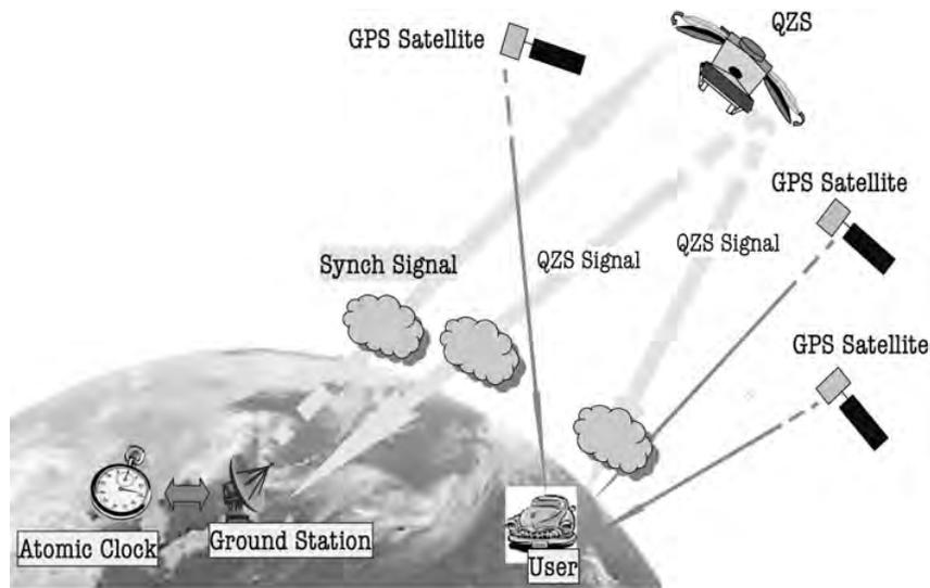
Figure 3.1: RESSOX system. The QZSS works as complementary system for the present GPS and also provides augmentation features.
