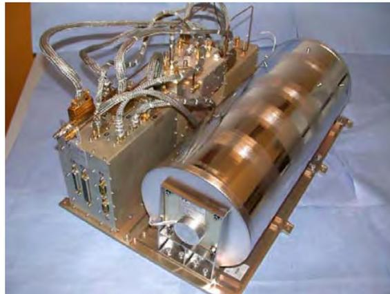
Figure 2.6: Engineering Model of GALILEO Passive Hydrogen Maser (PHM) atomic clock [36].
