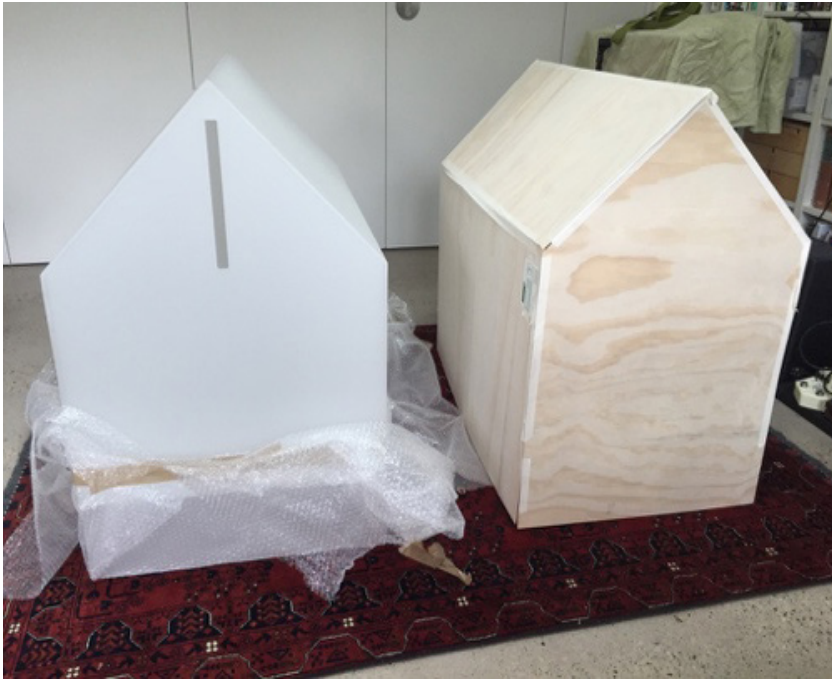
Figure 51: Maquette and fabricated house from acrylic sheet.
