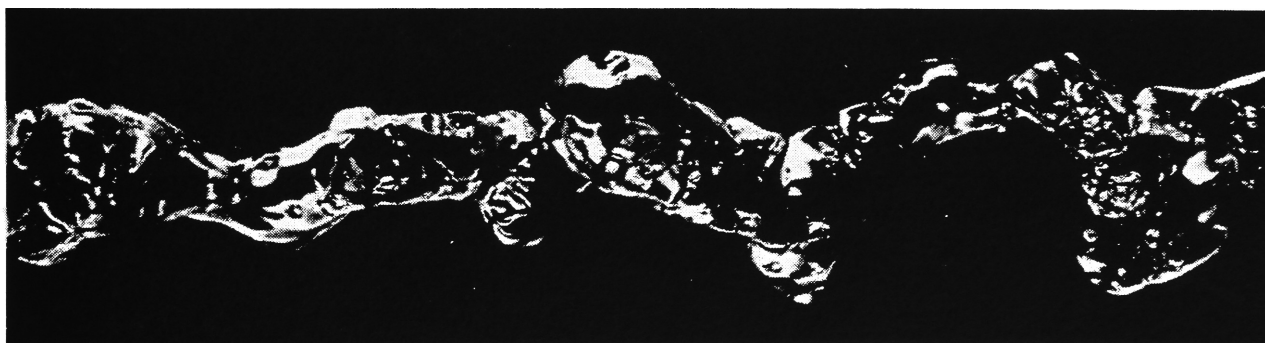
Figure 5. A jet displaying a helical instability - from plate 4 of Hoyt and Taylor (1977).
