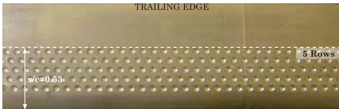
Figure F.2 Tyrrell026 Airfoil with 1.5-5-53 Series Dimple Array Modification
