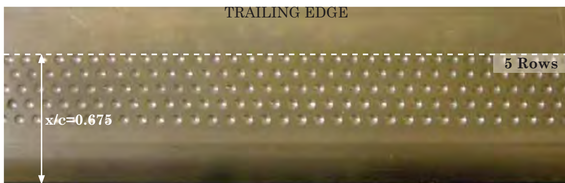
Figure F.3 Tyrrell026 Airfoil with 1.5-5-675 Series Dimple Array Modification
