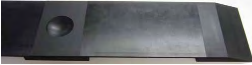
Figure 5.3 Single Dimple Test Model
