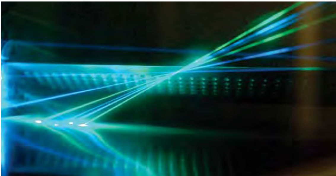
Figure 8.1 LDA Measurements in the Wake of a Dimpled Airfoil
