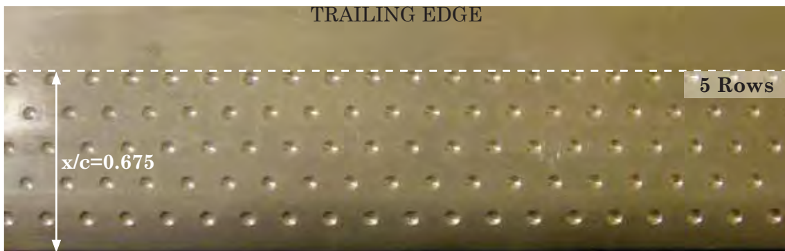
Figure F.9 Tyrrell026 Airfoil with 2.5-5-675 Series Dimple Array Modification
