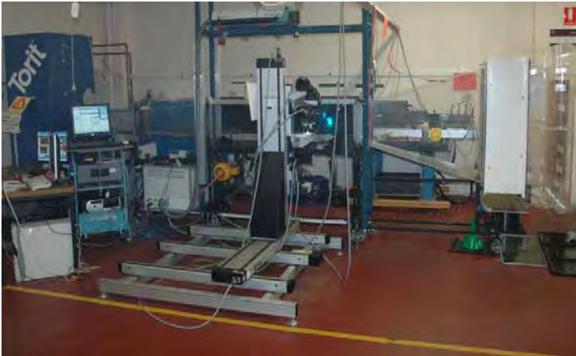
Figure 3.1 Wind Tunnel in Primary 'Moving Ground' Configuration
