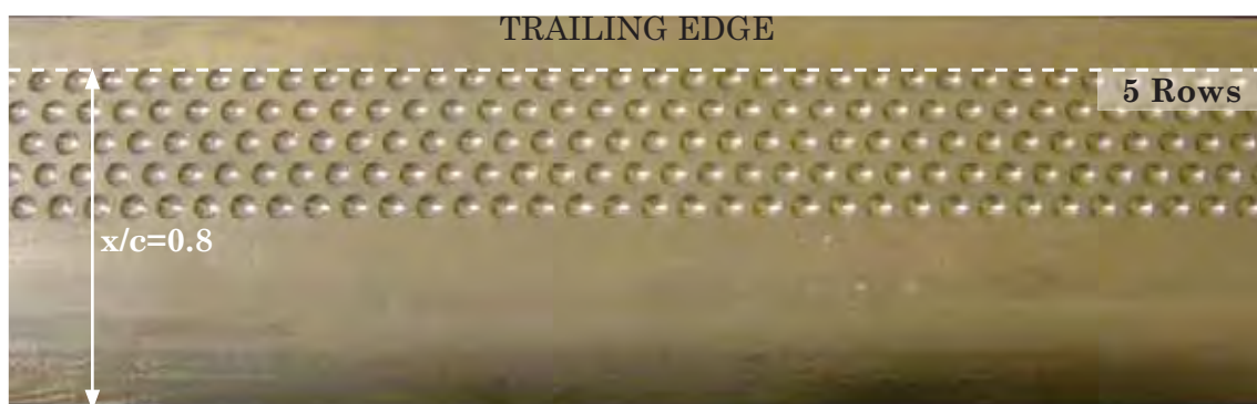
Figure F.4 Tyrrell026 Airfoil with 1.5-5-8 Series Dimple Array Modification
