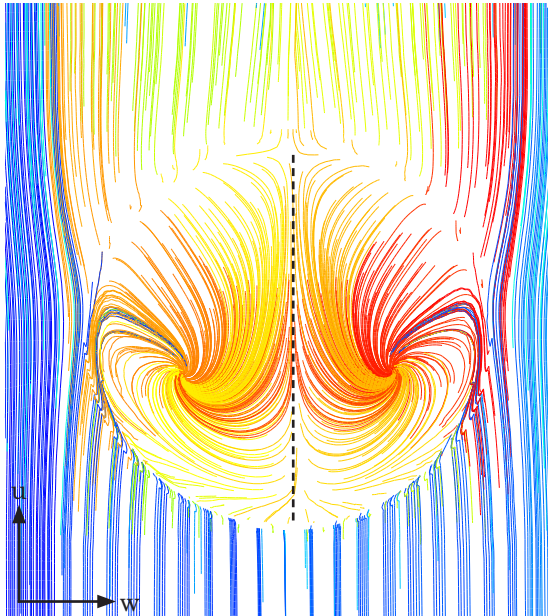
Figure 5.34 Surface Pathlines Re_D=4.3 \times 10^3 Coloured by Particle Position on Surface
