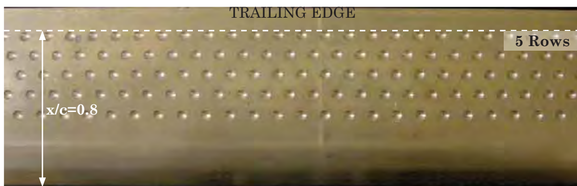
Figure F.7 Tyrrell026 Airfoil with 2-5-8 Series Dimple Array Modification
