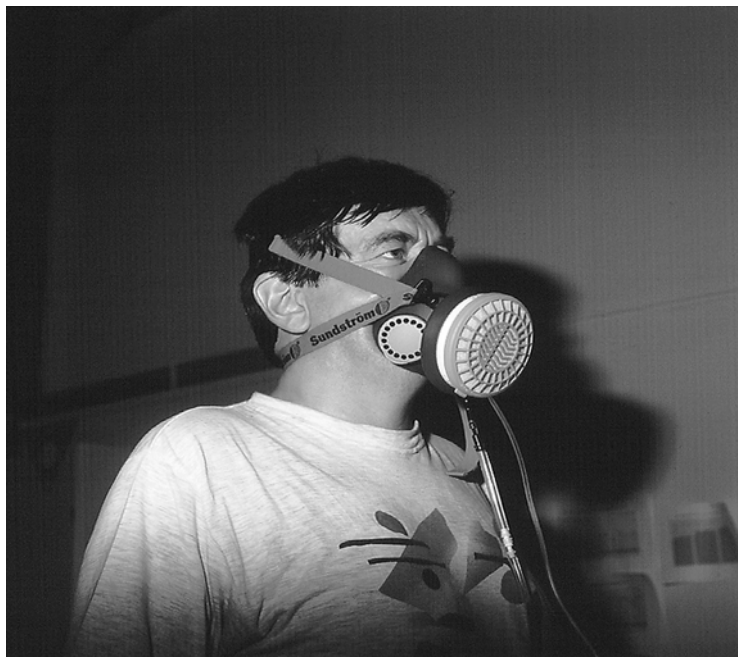
Figure 5.1: Close-up of half-face respirator used. The tubes allow the Pressure changes to be communicated to the measuring equipment.
