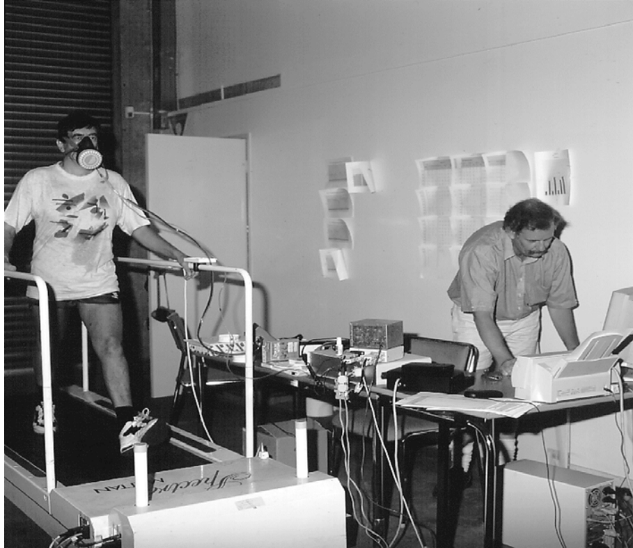
Figure 5.2: Photograph of a person exercising at a constant rate and the monitoring in the laboratory showing equipment used to determine minute volumes of air used by each volunteer
