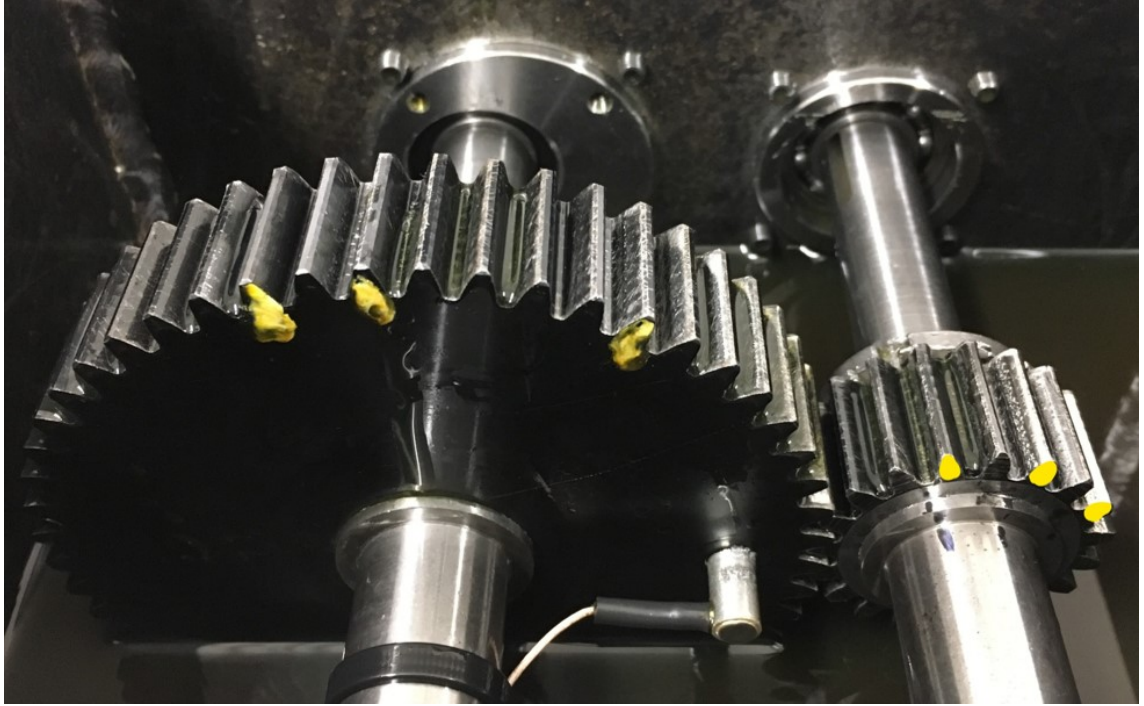
Figure 3.3: The pair of spur gears used in the lubricated test. The left is the driven gear and the right is the driving gear. The yellow marked teeth are the ones for moulds making during the test. The dry test used another gear pair with the same configuration and material.
