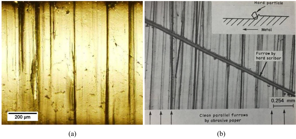
Figure 6.5: (a) A mould image of a gear surface subjected to abrasive wear in the lubricated test, (b) the reference in [232].
