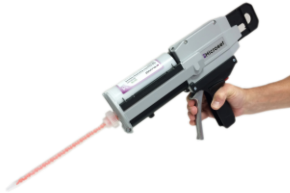
Figure 3.4: The replication compounds dispenser used in this research [181].
