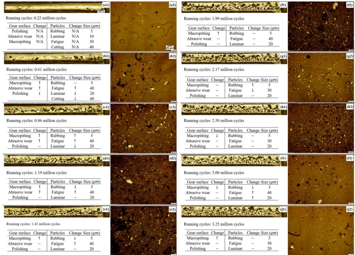
Figure 5.7: The evolution of gear macropits and wear particles. (a1) – (j1) mould images, (a2) – (j2) wear particle images. Texts summarise wear information, including running cycles, wear mechanisms on gear surface in the order of severity, their changes with respect to previous ones, wear particle types in the order of proportion, their changes with respect to previous ones, and approximate sizes. Note ‘↑’, ‘↓’ and ‘—’ means increase, decrease and no apparent change, respectively.
