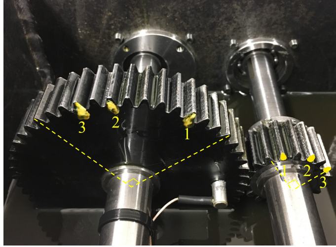
Figure 4.1: The driven (left) and driving (right) gears. The marked teeth were monitored continually using the method developed in section 4.2.2.
