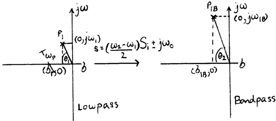
Fig. 3.4. Transformation from the lowpass filter to the bandpass filter ( consider a pole only)
