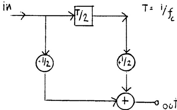
Fig. 4.8. Flowchart representation of the bandstop filter obtained from (4.6)
