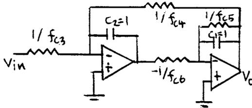
By assuming that  $C_1 = C_2 = C_6 = C_5 = C_3 = 1nf$  to simplify the calculation. We eventually get the bandwidth as demonstrated in (5.8)
