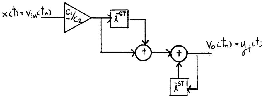
Fig. 2.13. A diagram of a sampled data system of Eq (2.38).
