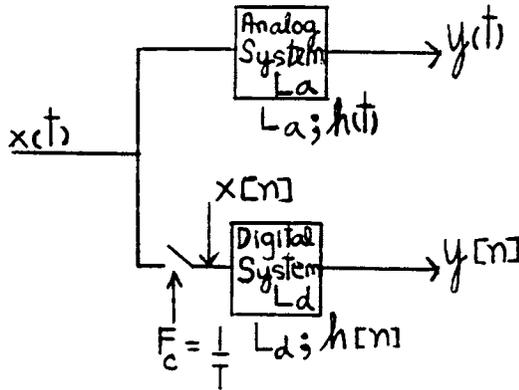
Fig. 2.1. Representation of a mixed analog ( $L_a$ )/simulated analog ( $L_d$ ) system.
