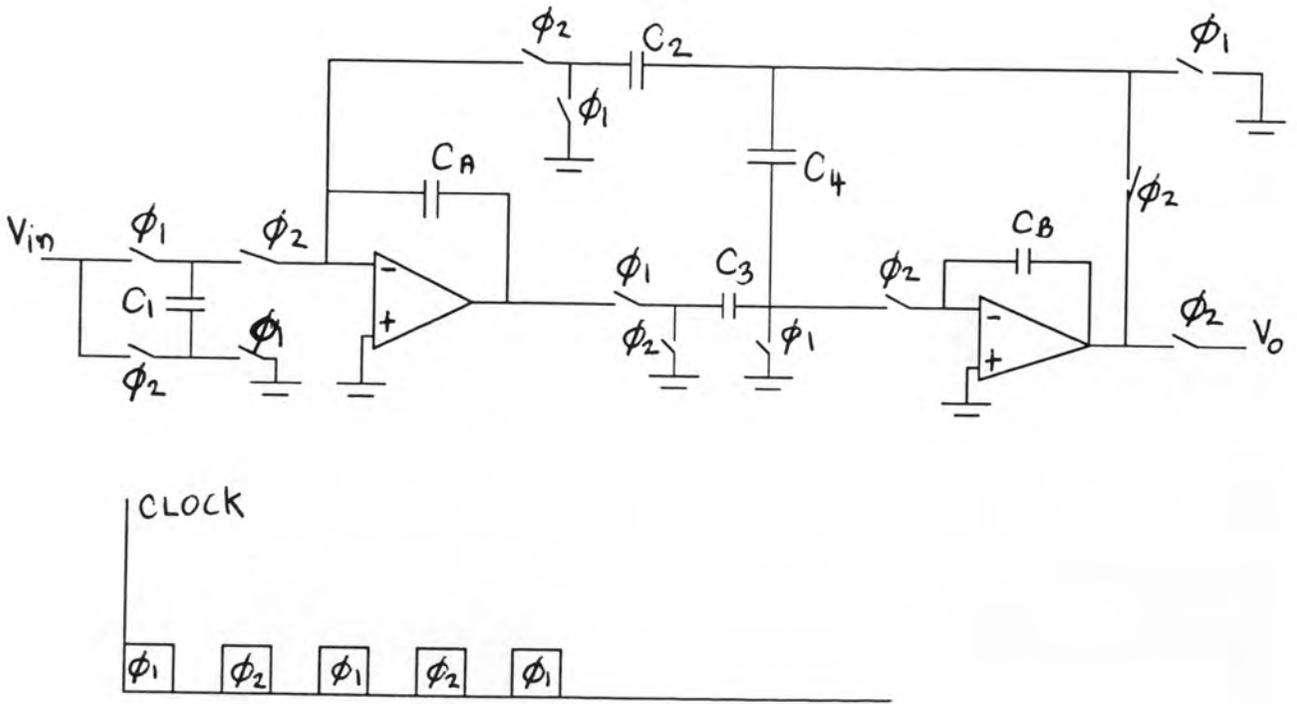
Fig. 6.1. A cosine decimation filter circuit.
