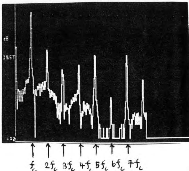
Fig. 6.21. The frequency spectra of the output of the interpolator ( $v_3$ )
