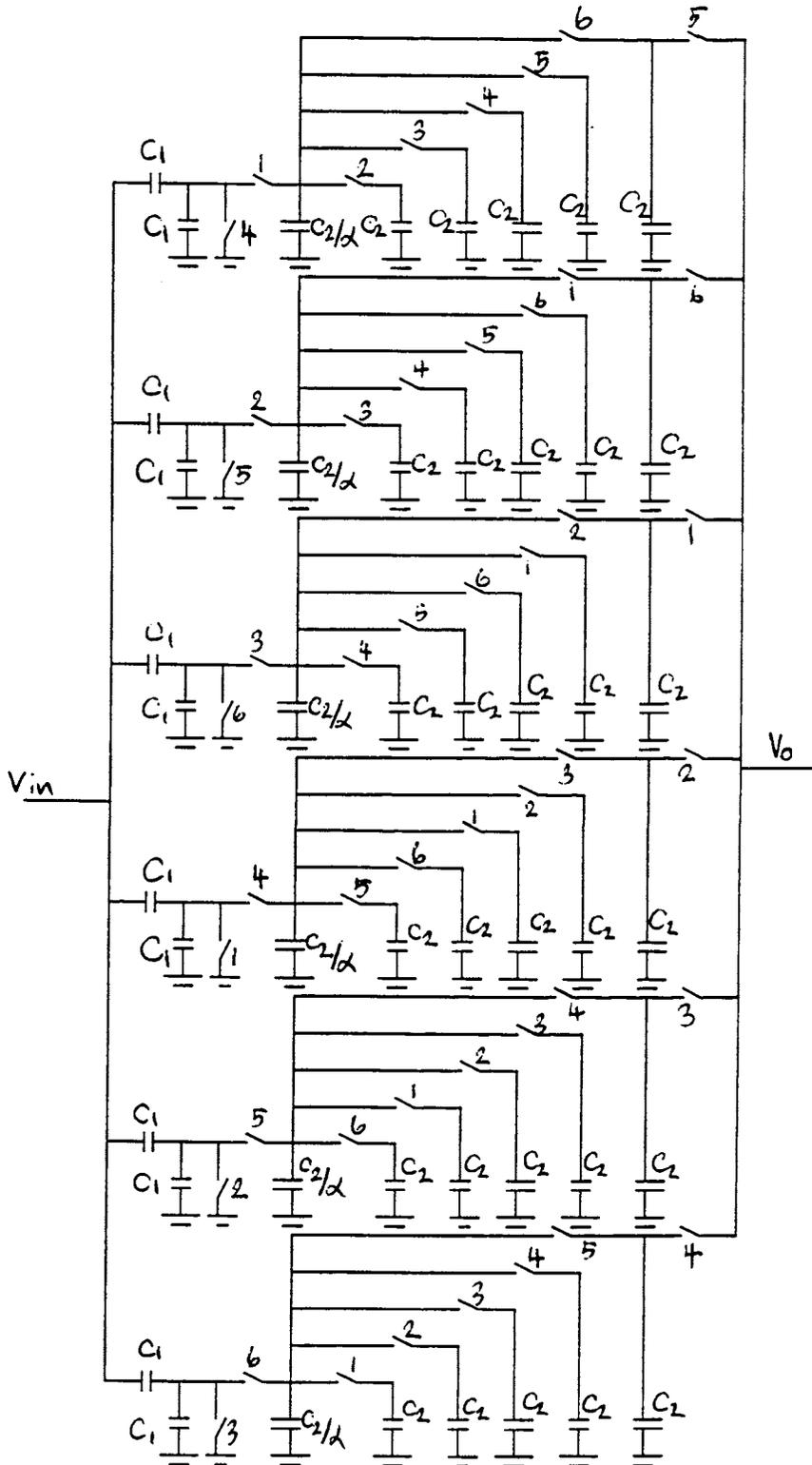
Fig. 6.7. bandpass switched-capacitor 6-path filter
