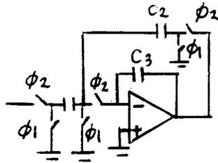
Fig. 5.10. A SC model which the switches are already reduced.
