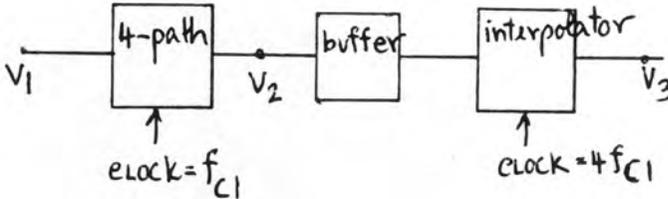
Fig. 6.15. The block diagram demonstrates the connection between the SC bandpass 4-path filter and the interpolator.
