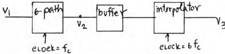
Fig. 6.18. The block diagram demonstrates the connection between the SC bandpass 6-path filter and the interpolator.
