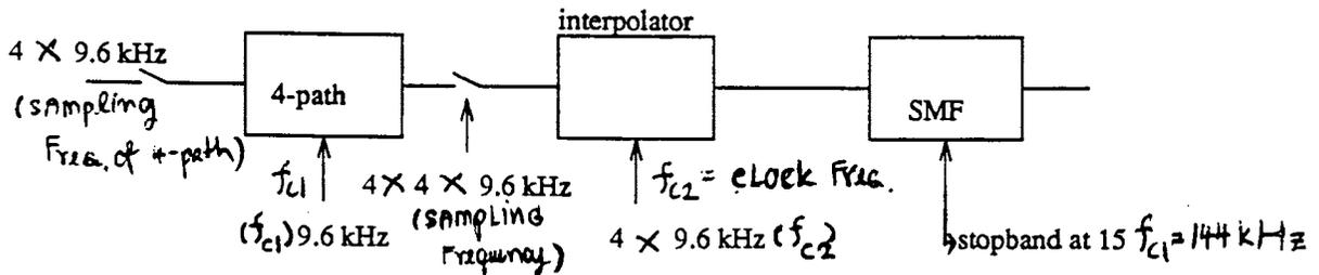
Fig. 6.27 Block diagram demonstrates the effective performance of interpolator to relax the specifications of smoothing filter
