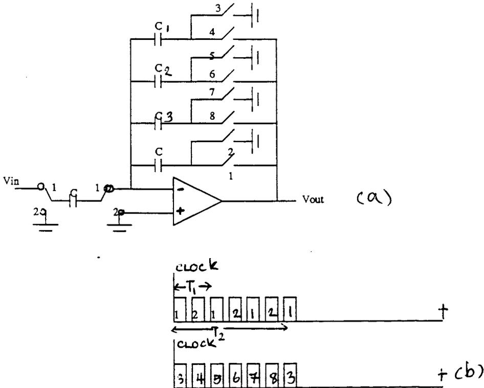
Fig. 4.17. Memory-type SC filter stage
