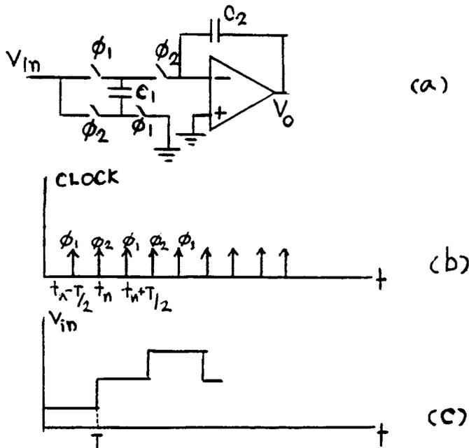
Fig. 2.12. (a) The switched capacitor integrator which simulates the operation of RC integrator by using bilinear transformation.
