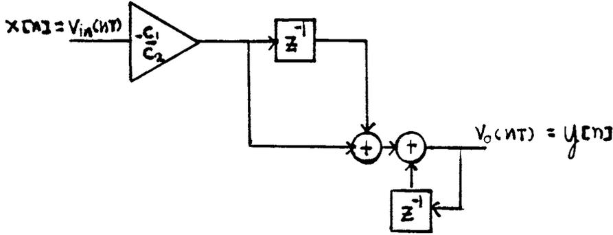
Fig. 2.14. A digital simulator of Fig. 2.13.
