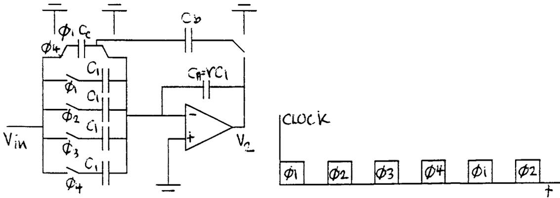
Fig. 6.12. An interpolation filter circuit
