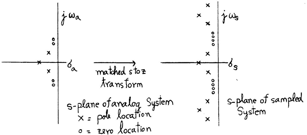
Fig. 2.4. (a) Locations of poles and zero of an analog system  $L_a$ .
