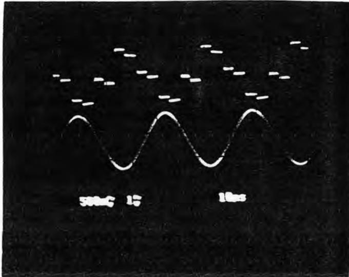
Fig. 6.5. A sampled and held output waveform (upper trace) and a sine wave input signal (lower)
