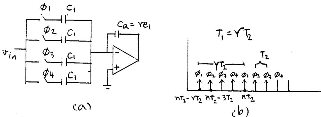
Fig. 5.21. An interpolation filter.
