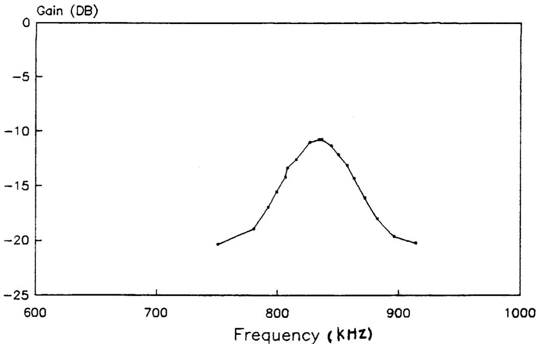
Fig. 6.11 The frequency response of switched-capacitor bandpass 6-path filter.
