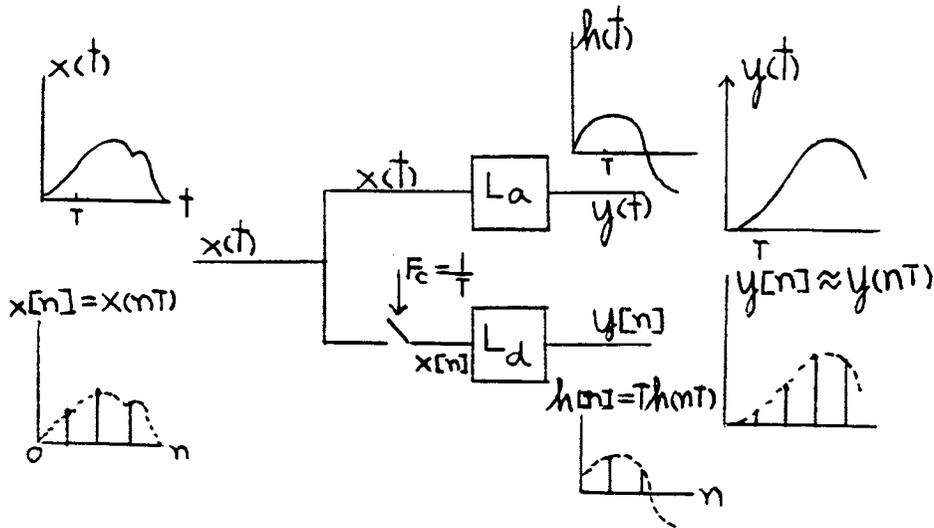
Fig. 2.2. Representation of a time sampling method of simulation.
