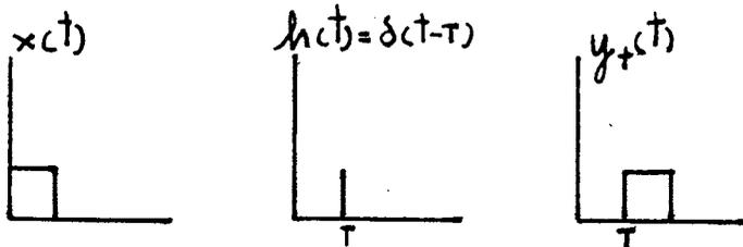
Fig. 2.11. A delay element of a sampled-data system.
