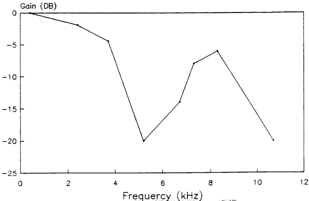
Fig. 6.13. The frequency response of the interpolator.
