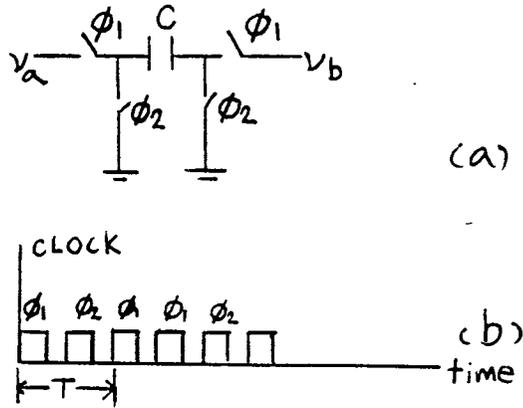
Fig. 1.1. a) Switched capacitor realization of a resistor branch.
