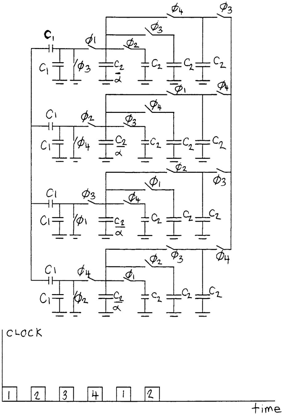
Fig. 4.11. A bandpass SC 4-path filter
