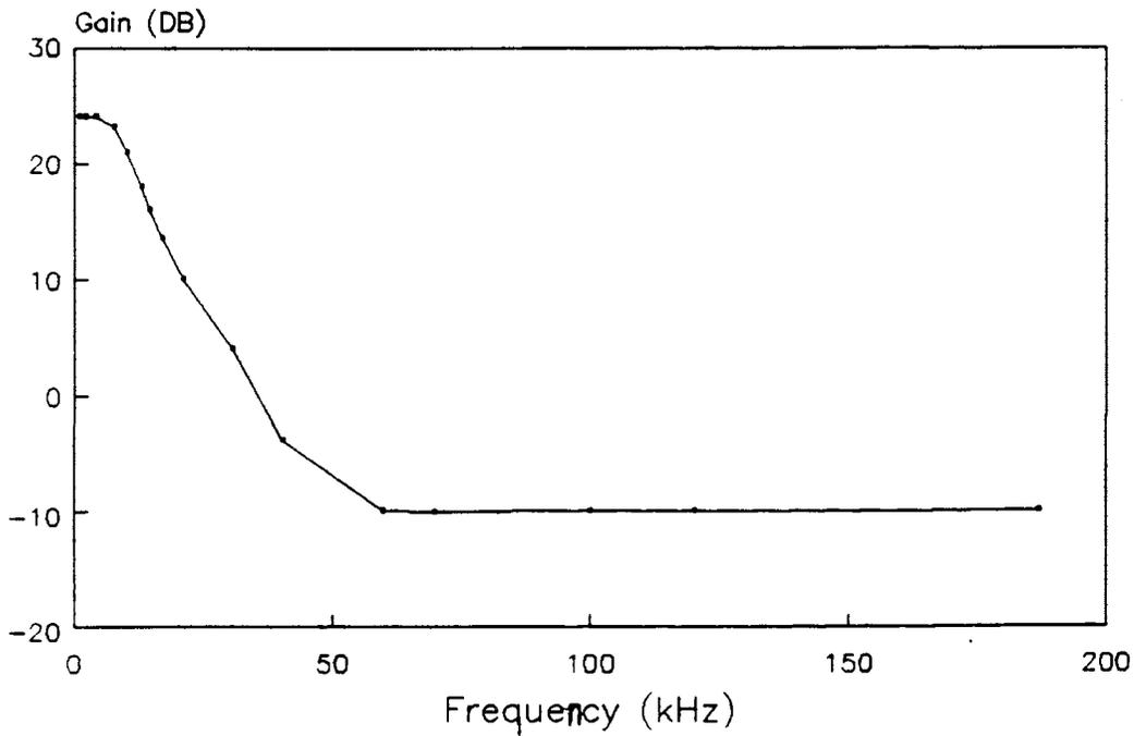
Fig. 6.3. The frequency response of the cosine decimator
