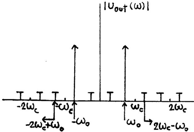
Fig. 4.2. N-path filter output spectrum containing spectral fractions of mirror frequencies.
