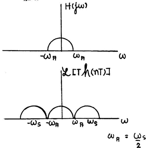
Fig. 2.3. (a) Frequency response of the transfer function of an analog system  $L_a$ .
