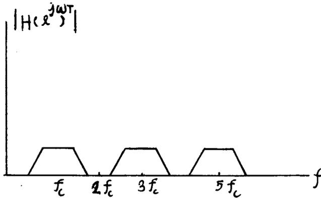
Fig. 4.10. The frequency response of prefilter.
