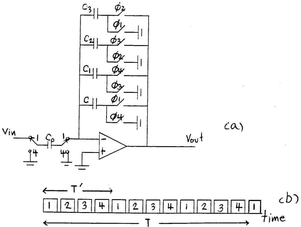
Fig. 4.16. Circulating-delay type pseudo-N-path filter stage
