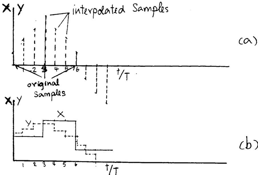
Fig. 5.18. (a) impulse-sampled signal
