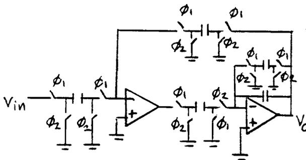
Fig. 5.8. A full switch model of a SC circuit which realises the biquadratic transferfunction.
