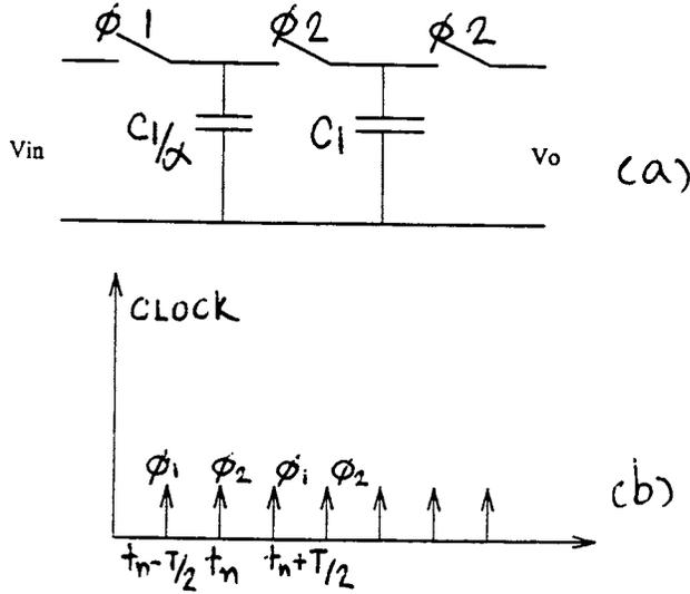
Fig. 4.3. a simple passive filter (a) circuit diagram (b) clock signals
