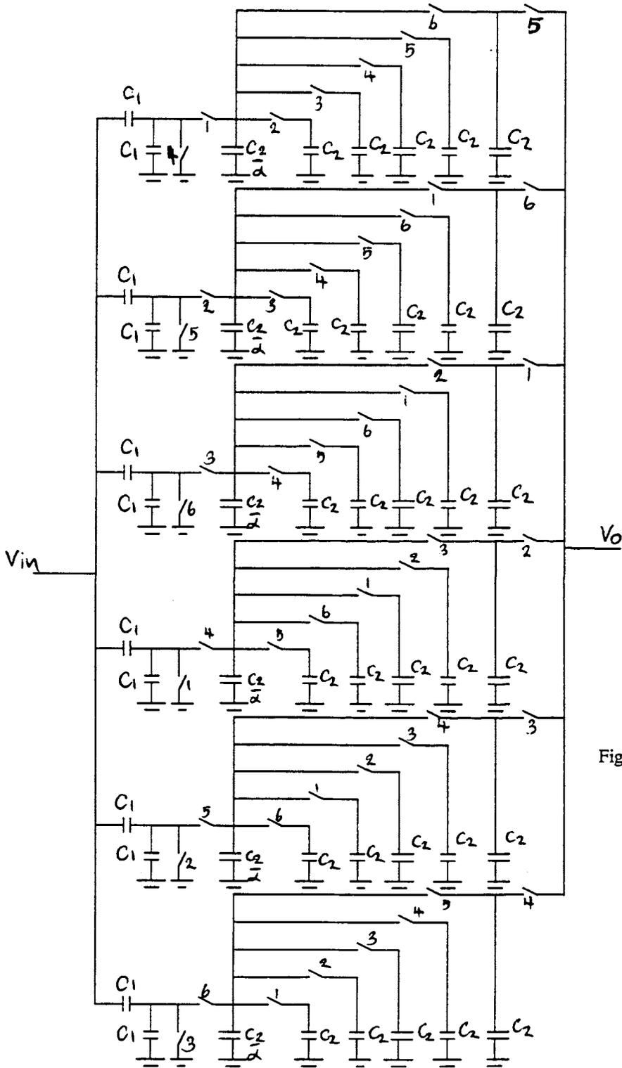
Fig. 4.13. The SC bandpass 6-path filter
