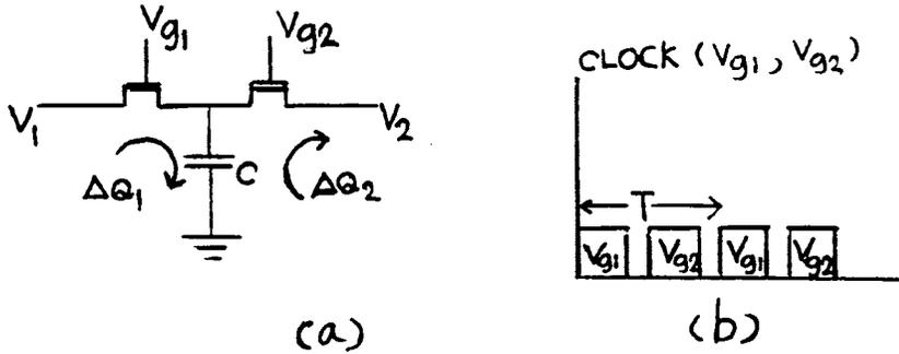
Fig. 3.1. (a) Representation of a switched-capacitor simulator of a resistor.
