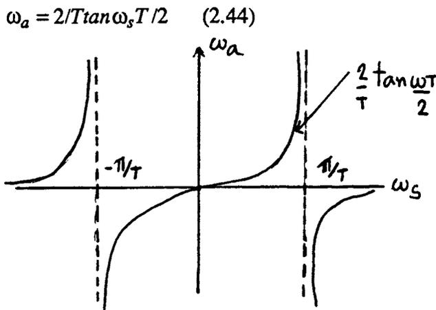
Fig. 2.16. The relation between the continuous-time and sampled-data frequencies for the bilinear s to z mapping.
