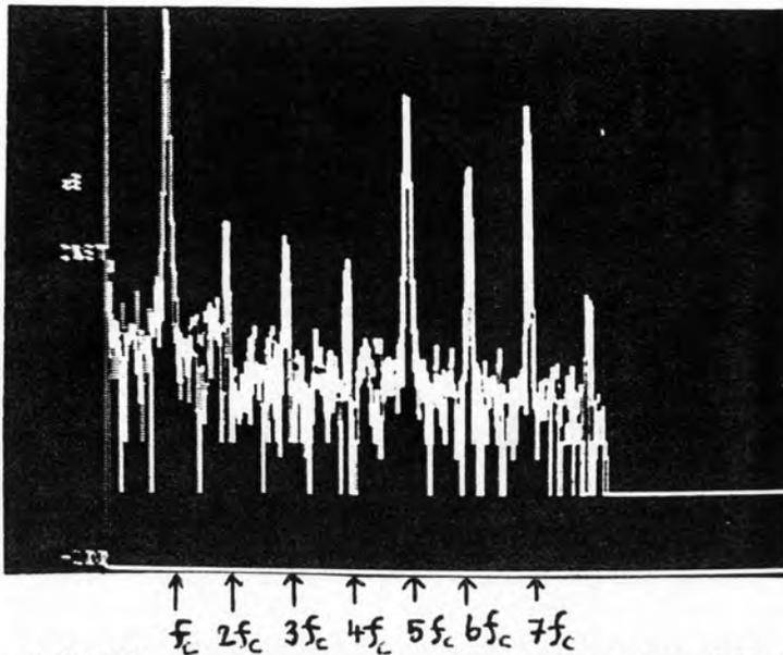
Fig. 6.20. The frequency spectra of the output of the SC bandpass 6-path filter.
