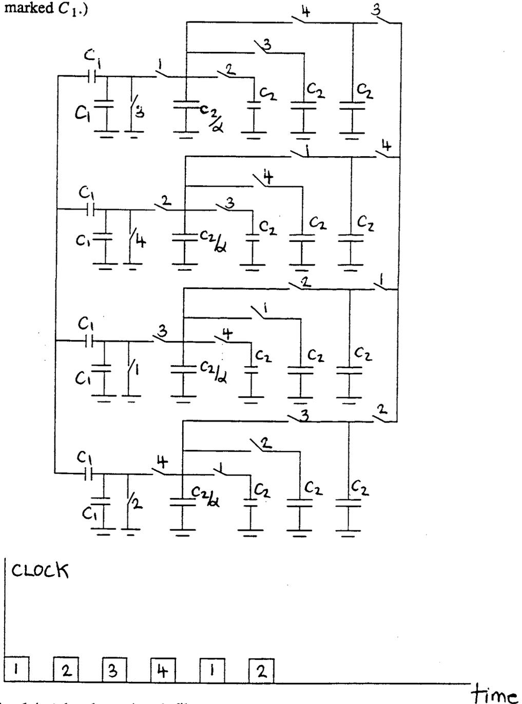
Fig. 6.4. A bandpass 4-path filter.
