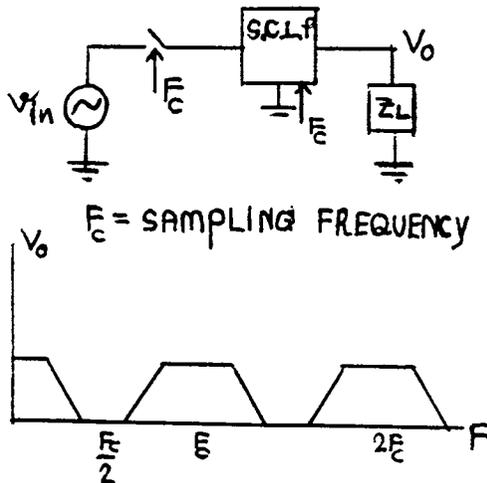
Fig. 3.5. Amplitude response of the SC lowpass filter (Asclp).
