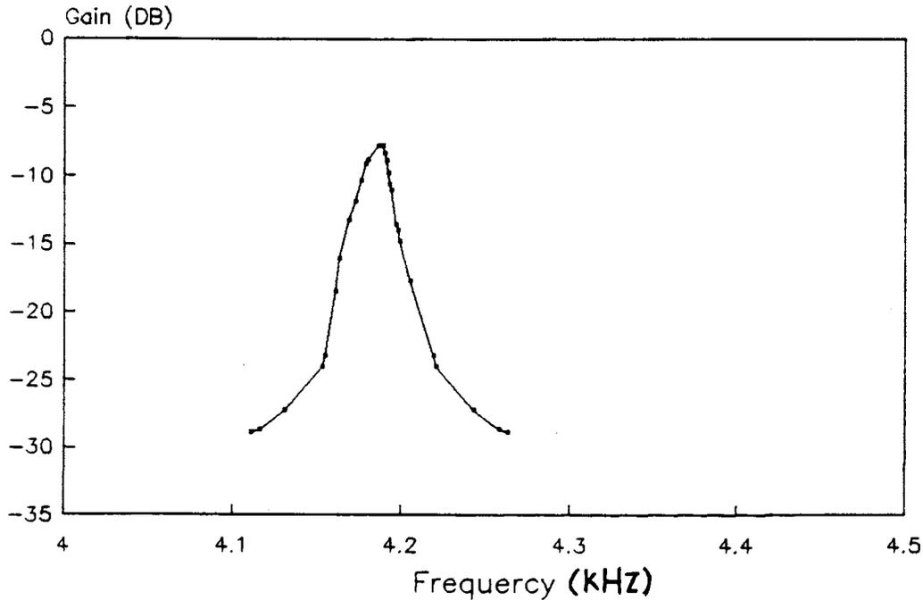
Fig. 6.6. Frequency response of the SC bandpass 4-path filter
