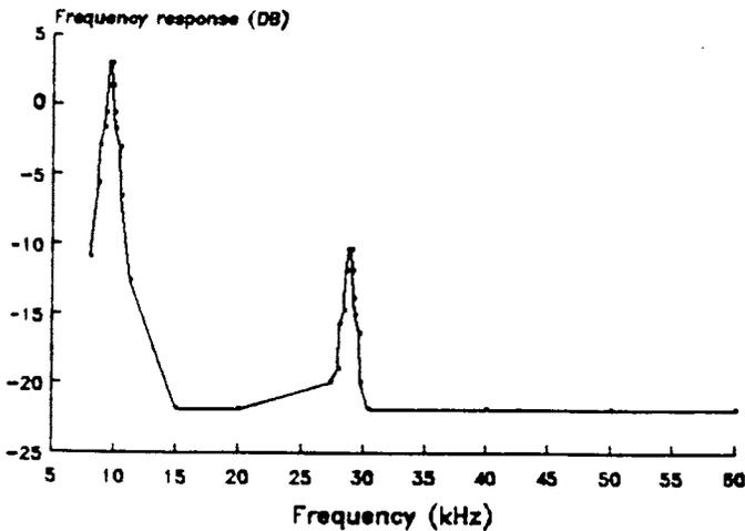
Fig 6.25 Frequency response of  $\frac{v_5}{v_{in}}$ .
