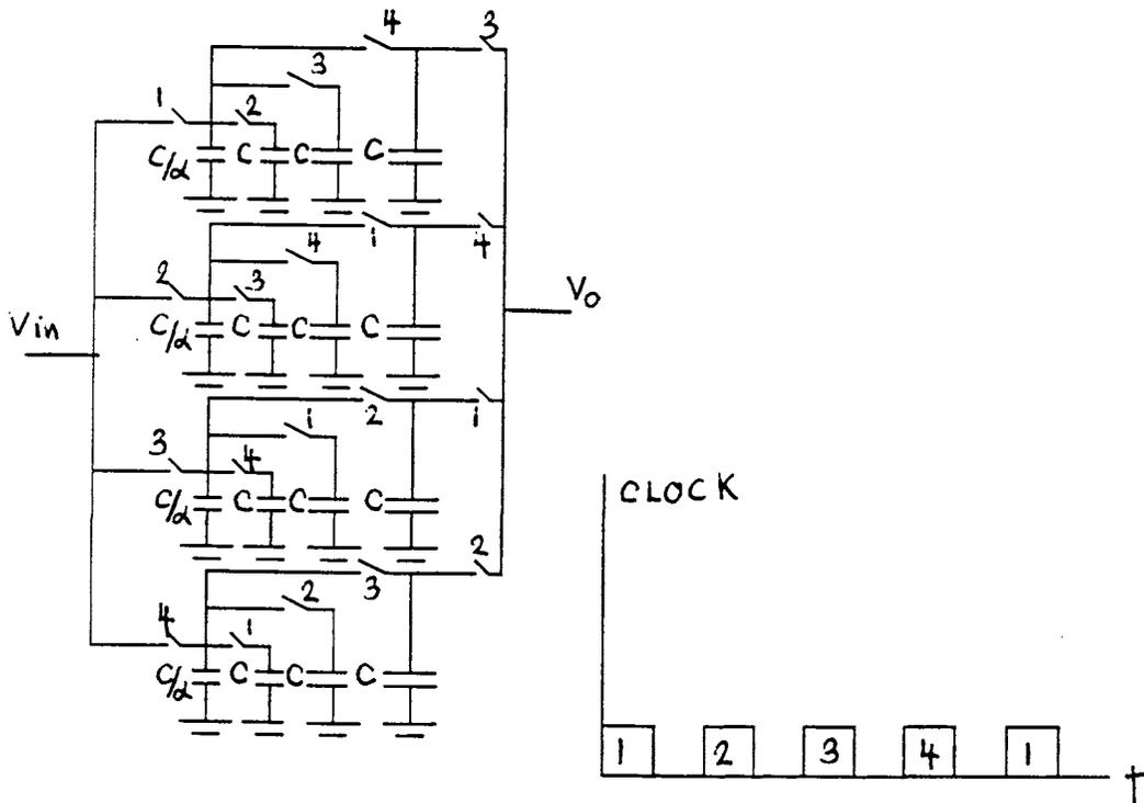
Fig. 4.7. Passive 4-path filter.
