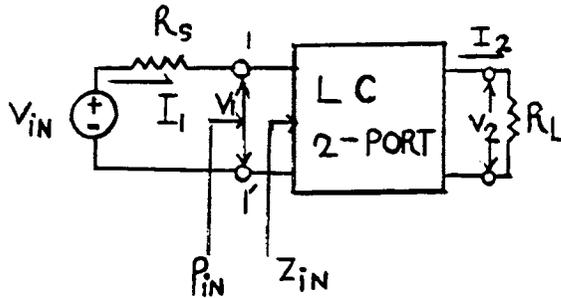
Fig. 3.2. Representation of a doubly terminated reactance two port with generator impedance  $R_s$  and load  $R_l$ .
