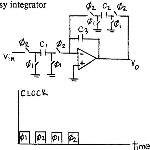
Fig. 5.9. A full switch model of a RC integrator
