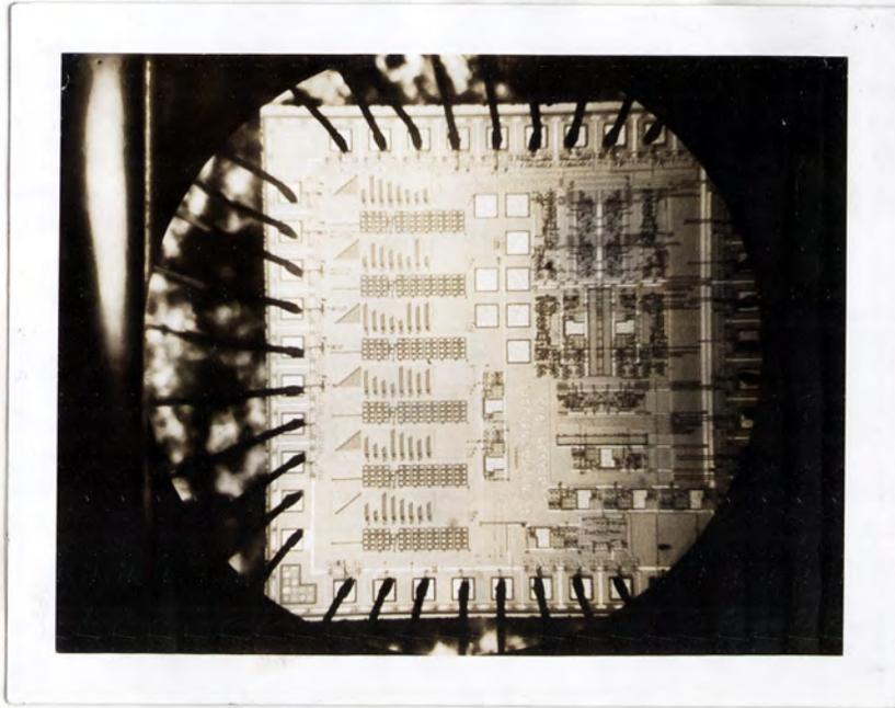
Fig. 6.8. The layout diagram of a switched capacitor bandpass 6-path filter
