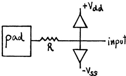
Fig. 6.10 The input protection circuit.
