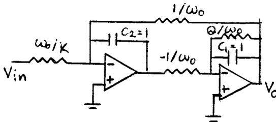
Fig. 5.6. Circuit diagram of a biquadratic transferfunction
