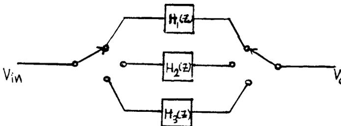
Fig. 3.6. Representation of 3-path filter.
