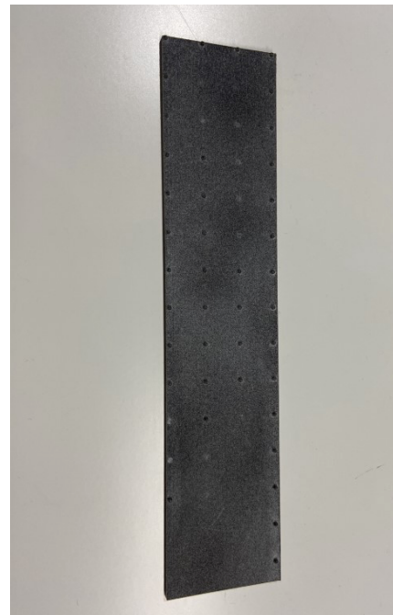
Figure 2-4 Examples of the 2 dominant spacer types in FO processes a) a woven spacer type with glue line in the middle and b) a segment of the 'dot spacer' design used in FO.
