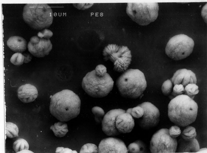
PLATE B2 PE8 Vaterite and the very rare acicular aragonite entity found in this experiment, 1000x magnification.
