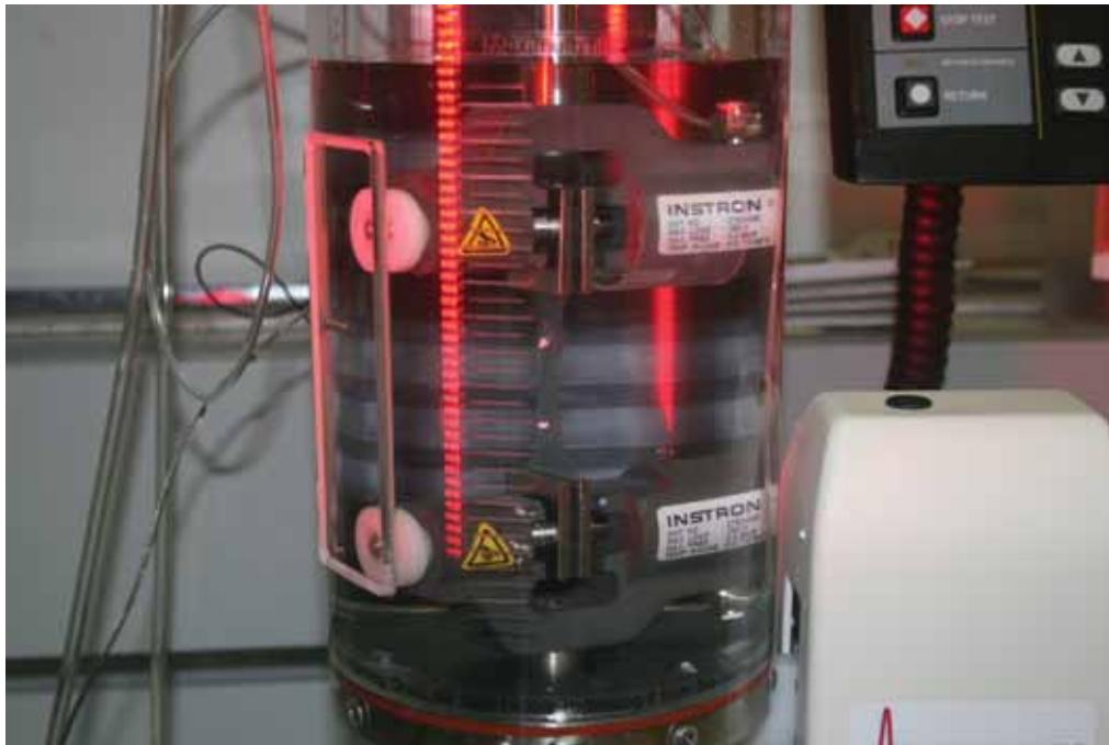
Figure L.1: 10% gelatine test setup. Note that the upper grip is fitted with a sleeve to prevent the air bubble build-up artifact
