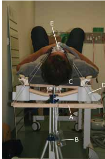
(b) Gravitational headgear tensioning. A) Spreader bar, B) Calibrated masses and suspension containers, C) Head support, D) Tension only cables loading headgear, E) CPAP mask
