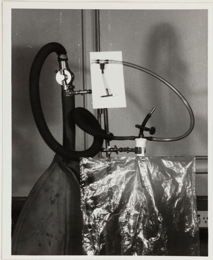
Figure 22. Apparatus for administration of oxygen mixtures.
