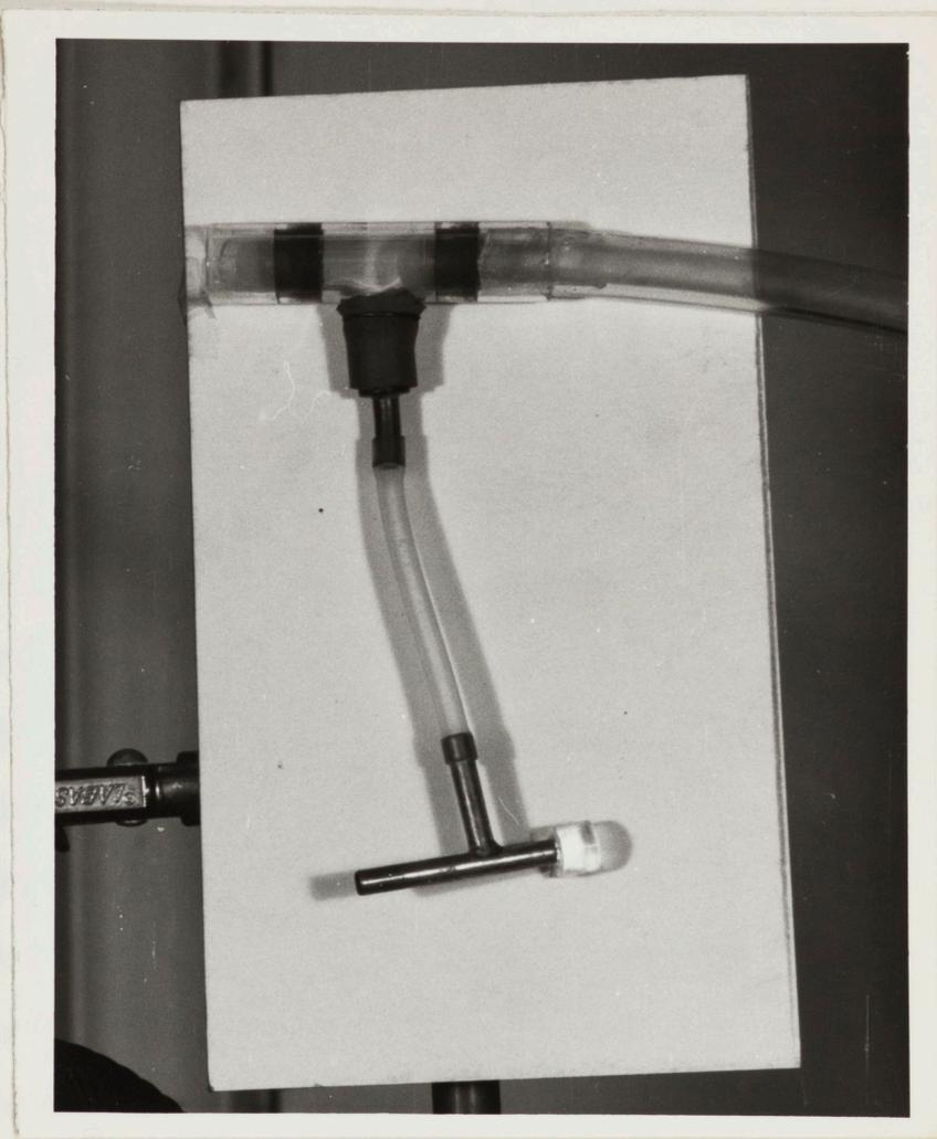
Figure 23. Details of respiratory valves and tracheotomy tube. The flap of the inspiratory valve is in the open position.
