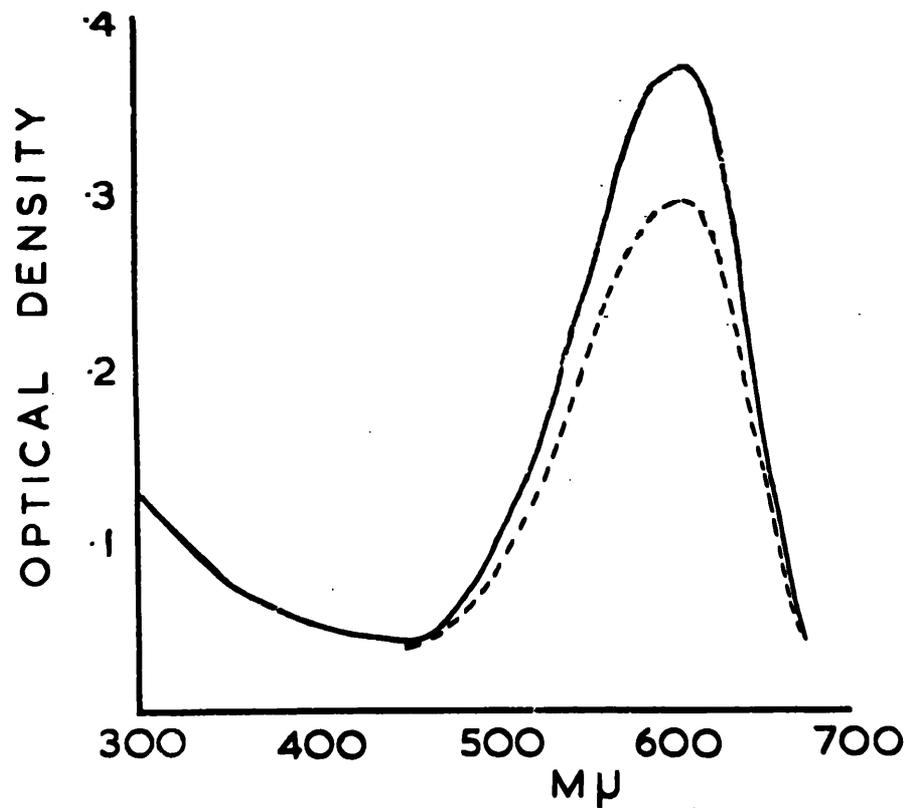
Figure 19. Calibration curves for the dye T-1824 in 0.9% saline (open circles) and in plasma (black circles).
