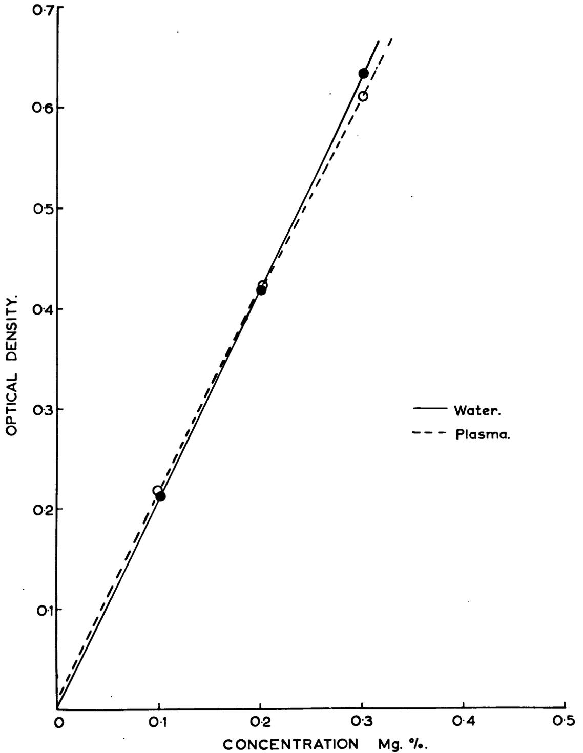
Figure 16. Calibration curves for the estimation of creatinine in water and plasma. Concentration of creatinine in plasma is expressed as mg per 100 ml of protein-free filtrate. Optical density measured at 520 m $\mu$ .
