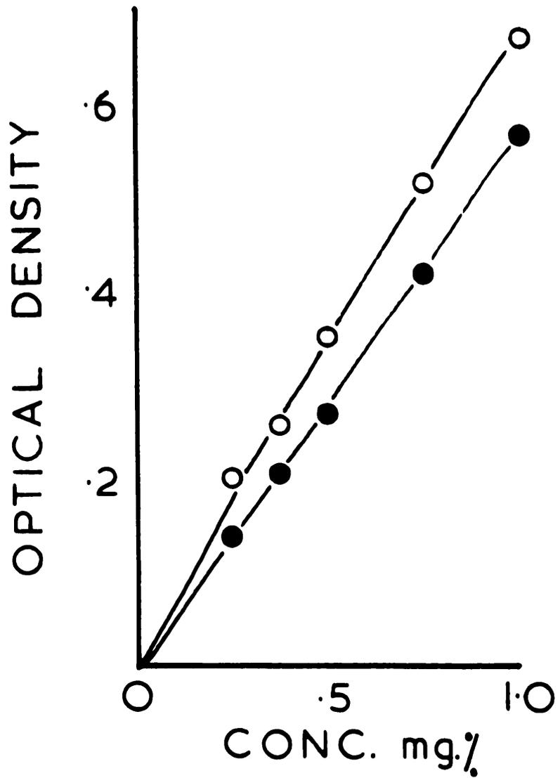
Figure 19. Calibration curves for the dye T-1824 in 0.9% saline (open circles) and in plasma (black circles).
