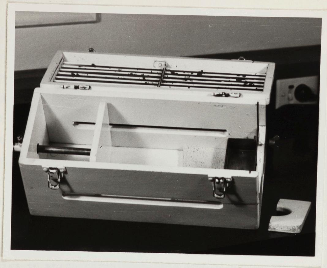
Figure I. Rabbit box with lid open and headpiece removed. Partition can be slid back to allow animal to sit with its head inside the box.
