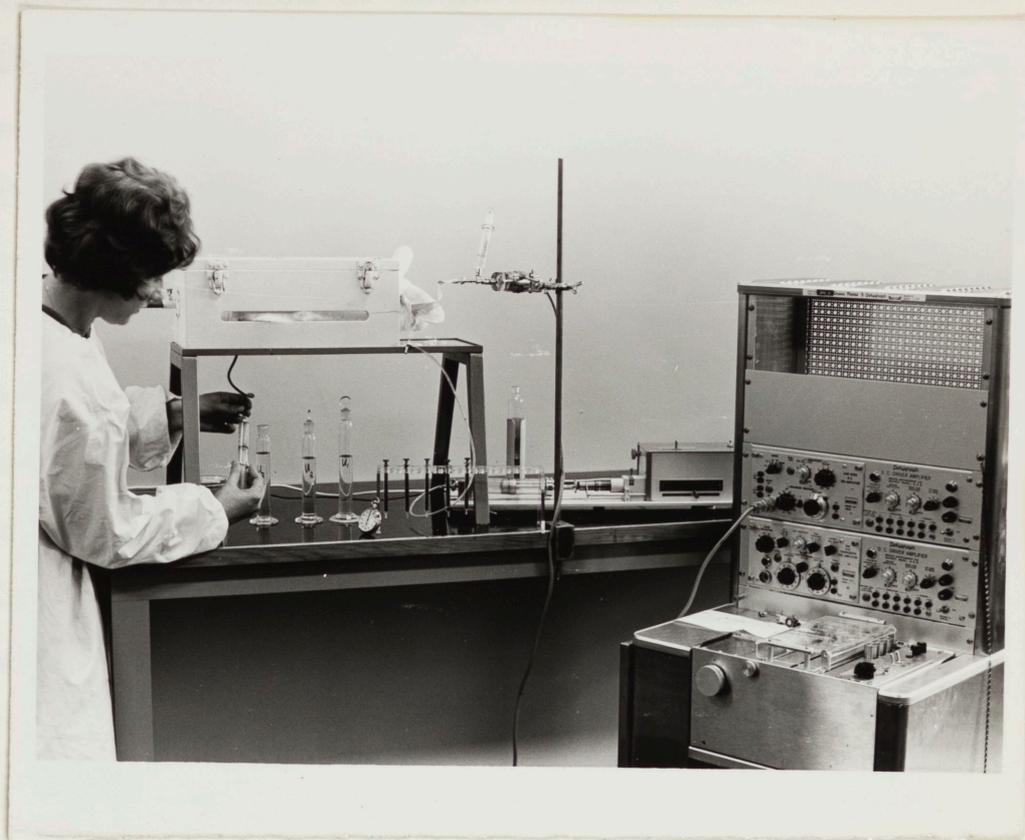
Figure 10. Apparatus used in measurements of renal clearance and blood pressure, showing infusion pump, blood-sampling syringes, pressure transducer and polygraph. A urine collection is being completed by irrigating the bladder with normal saline. In other experiments, in which the ureters were catheterized, the catheters were brought through the slits on either side of the rabbit box.
