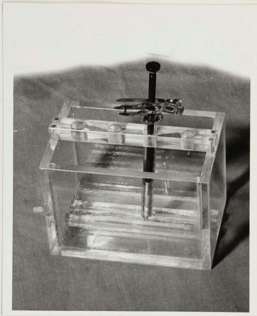
Figure 24. Perspex bath for storing blood samples in ice.
