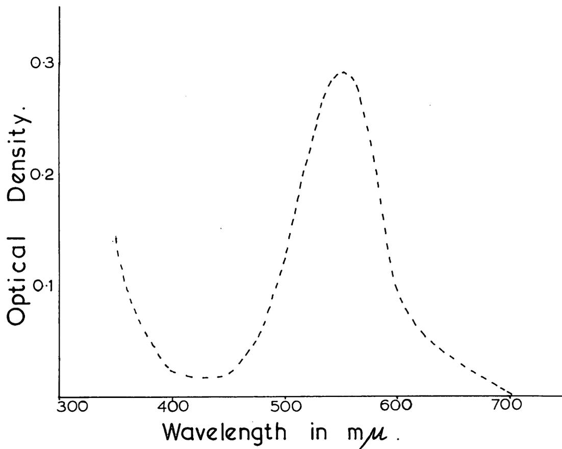
Figure 13. Absorption curve for PAI estimation.
