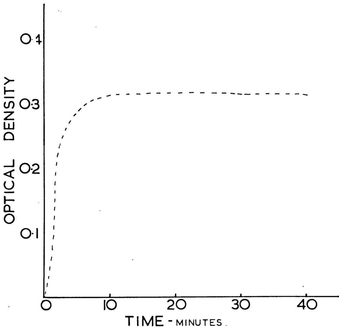
Figure 12. Rate of colour development after completion of coupling reaction at  $0^{\circ}\text{C}$ , in the estimation of sodium para-amino hippurate. Optical density was measured at 540 m $\mu$ .
