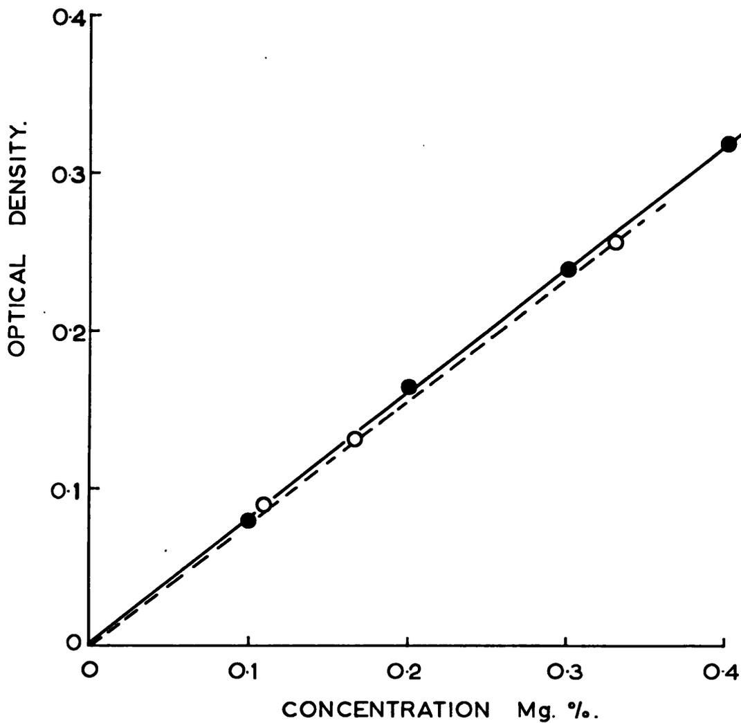
Figure 17. Calibration curves for the estimation of inulin in water and plasma. Concentration of inulin in plasma is expressed as mg per 100 ml of protein-free filtrate. Optical density was measured at 490 m $\mu$  (Smith, 1956).
