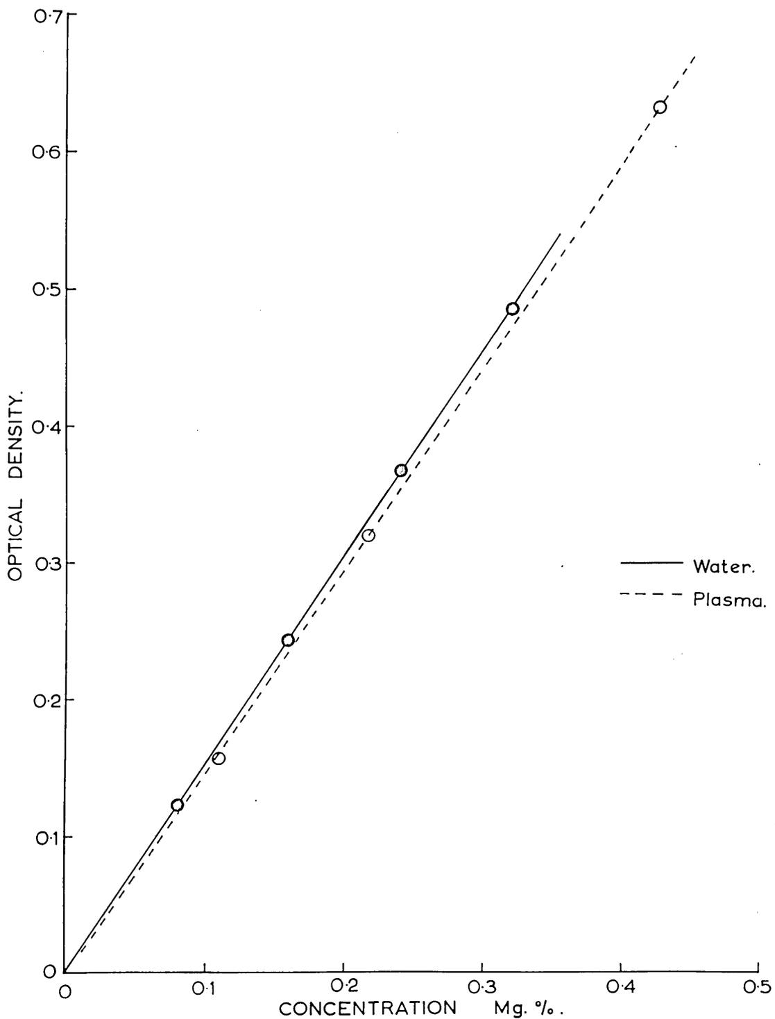
Figure 14. Calibration curves for the estimation of PAH in water and in plasma. PAH concentration in plasma is expressed as mg per 100 ml of protein-free filtrate. Optical density was measured at 540 m $\mu$ .
