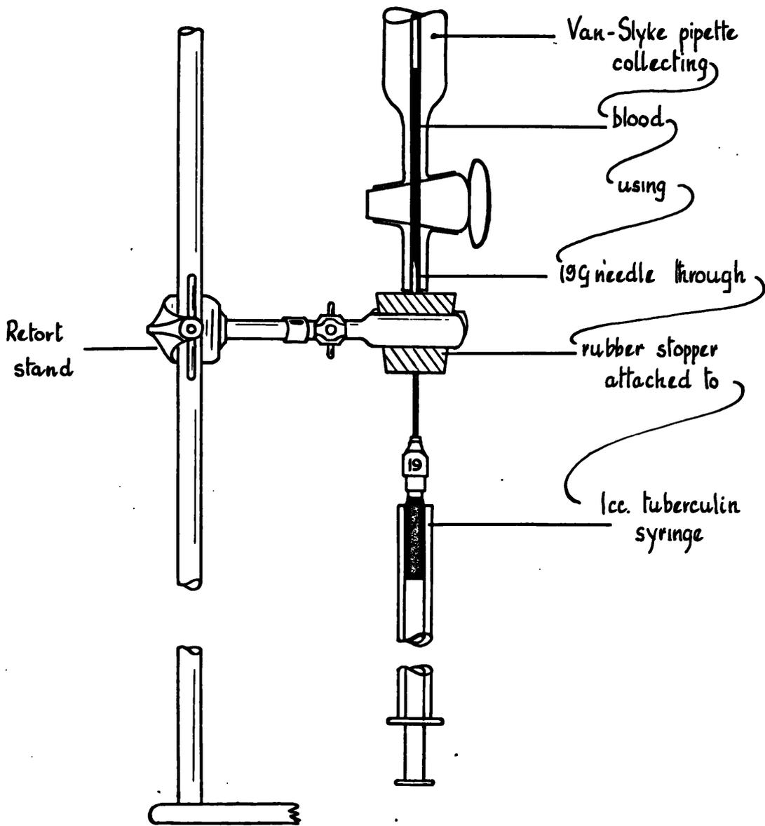
Figure 26. Transferring blood sample to Van Slyke pipette.
