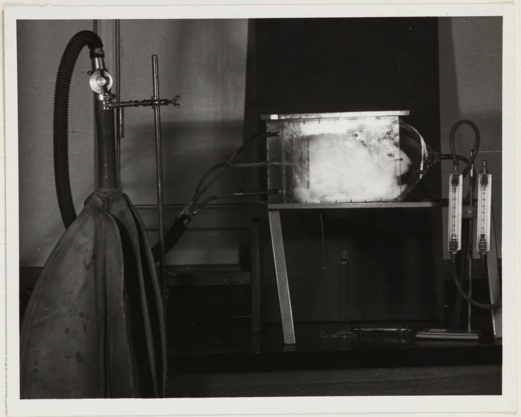
Figure 21. Apparatus for administration of carbon monoxide mixtures.
