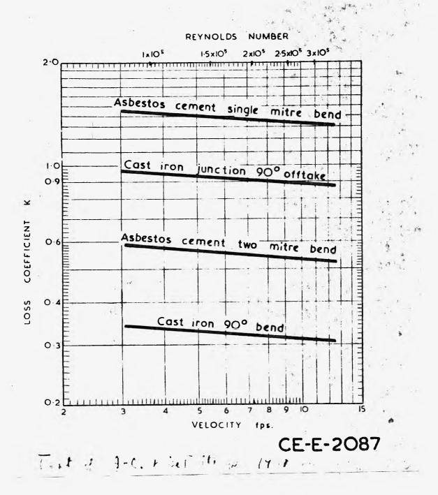
Fig 1. Loss coefficients of 4 in. fittings for asbestos cement pipes.
