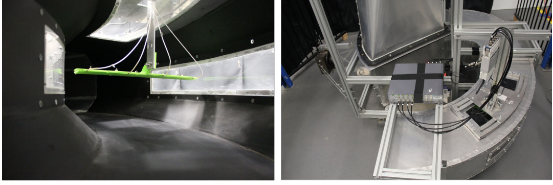
FIGURE 6.15: Position of hot-wire rake within test section and data acquisition system mounted externally
