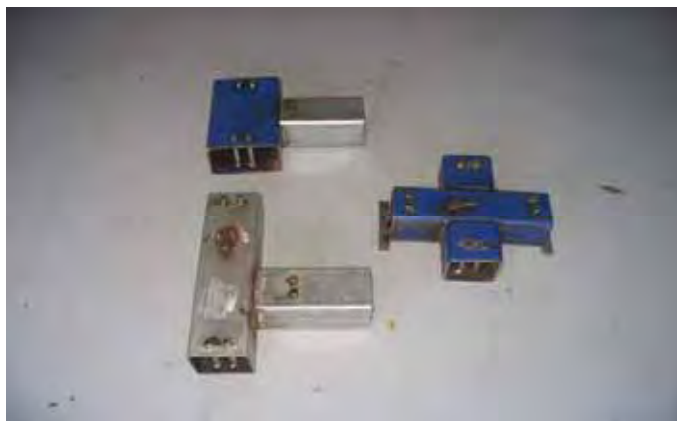
Figure 4.63c Jigs for bolt connection to lower C-brackets in internal of level 28.
