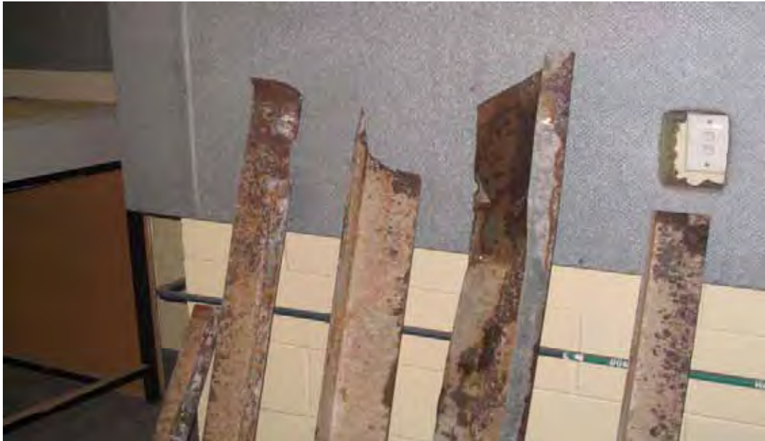
Figure 4.10 Sheet metal beneath the baffles and enveloping aluminium louvre panels, resulting in crevice corrosion on level 28 at corner of northern section closer to southern side.
