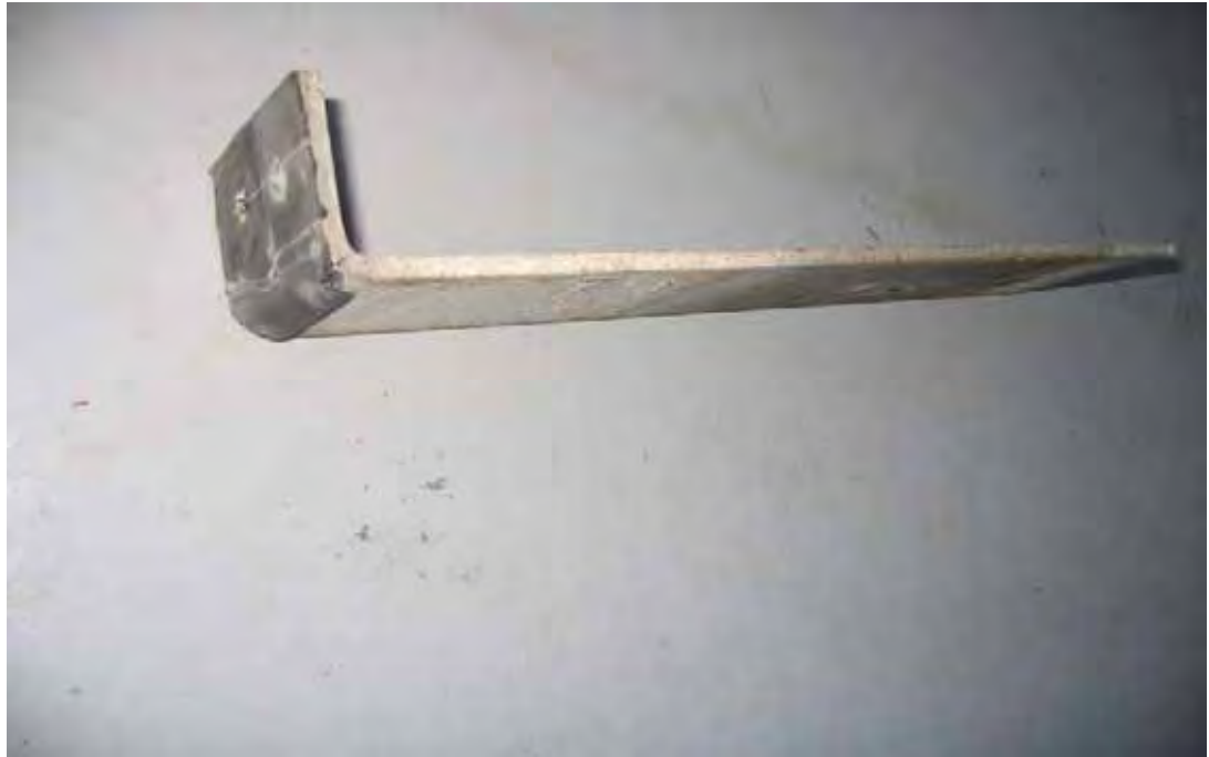
Figure 4.27 Rounded old brackets with cracks at radius.
