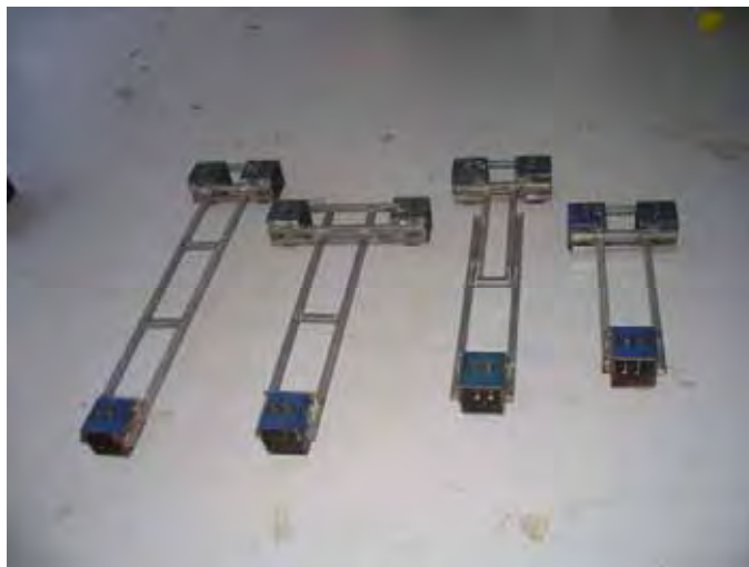
Figure 4.63b Jigs for bolt connection to upper U-brackets in internal of level 28.
