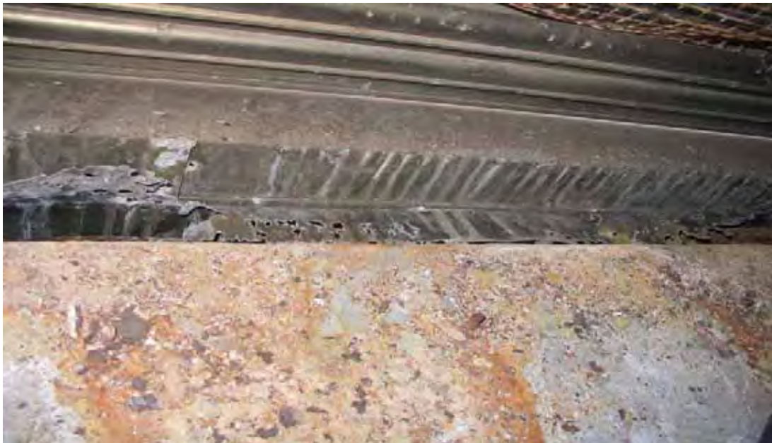
Figure 4.11 Aluminium panel section showing crevice corrosion and pitting corrosion owing to sheet metal coverage of aluminium.
