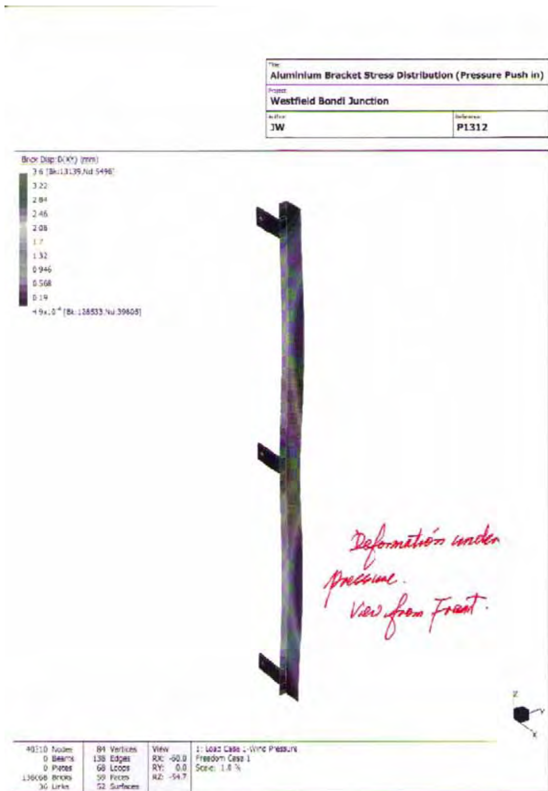
Figure 7.9 FEA illustrating buckling due to pressure forces, viewed from face of louvres.
