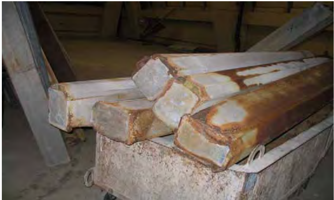
Figure 4.18 Excessive corrosion in baffles in open area of level 28, caused as result of moisture retained in fibreglass.
