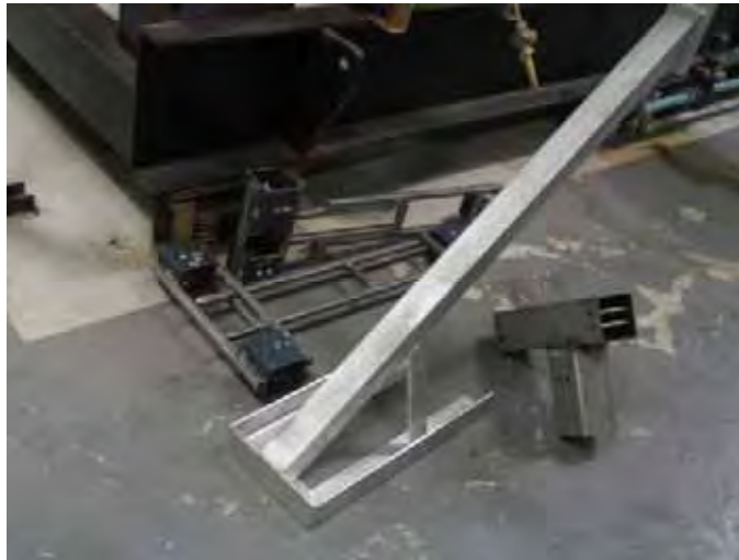
Figure 4.63a Special jigs engineered to allow marrying up of bolts from outside of mullions to connect through to internally fabricated brackets.
