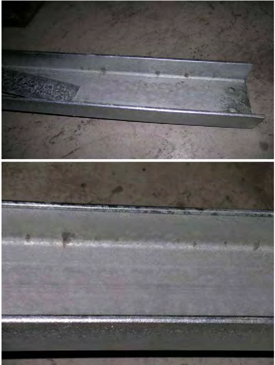
Figure 4.32 Chips of galvanised surface removed.
