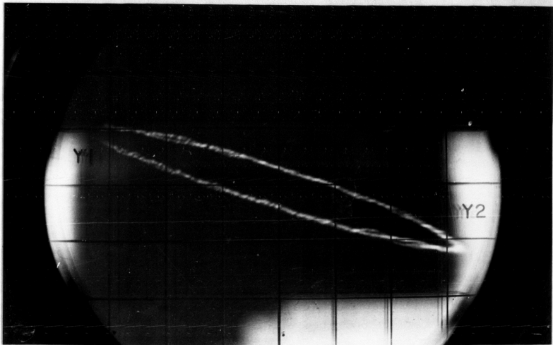
Fig. 25. Lissajous' figure, \Delta f = 0.5 MHz, r = 80 feet.
