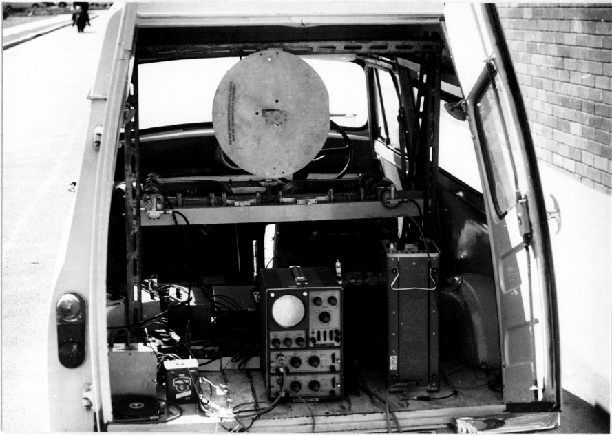
Fig. 36. Radar shown in the van. The Lissajous' figures were obtained on the oscilloscope facing the camera. The oscilloscope, with its axis vertical, to the right of the picture, was used to monitor the difference frequency.
