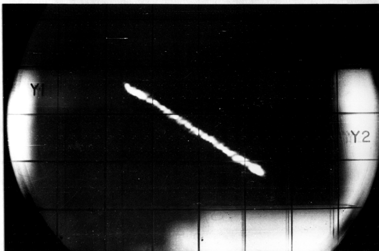
Fig. 26. Lissajous' figure, \Delta f = 0.5 MHz, r = 120 feet.
