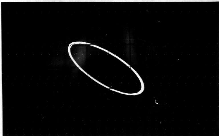
Fig. 20. Lissajous' figure, \Delta f = 1.5 MHz, r = 40 feet.
