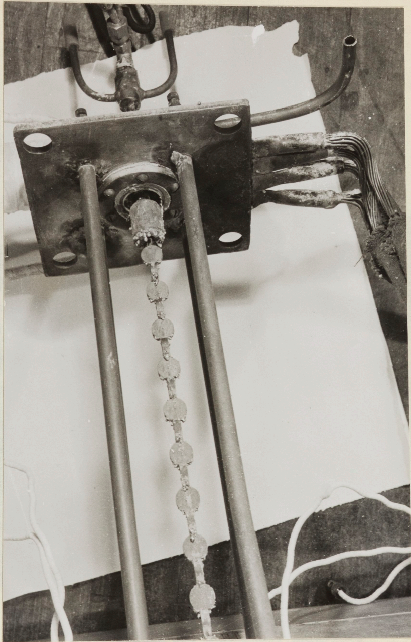
Fig. 9.7 - Photograph of Discs and Top Cover Plate showing Lead Splash around the Liquid Feed Nozzle
