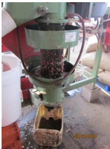
Figure 2.7 Mechanical demucilaging process
