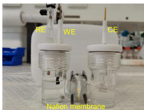
Figure 2.4 Photo of the standard three-electrode system in PEM H-Cell
