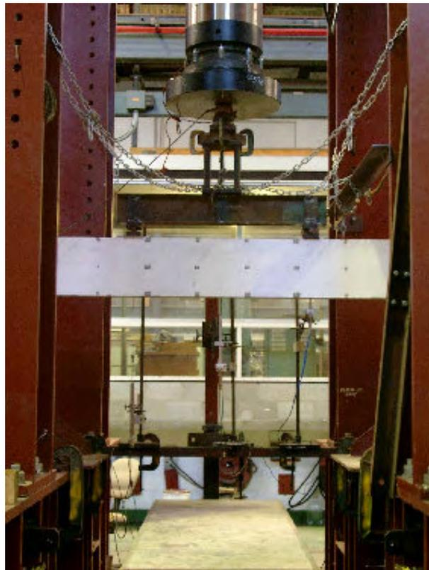
**Figure 3.11:** Test set-up for ultimate moment capacity tests
