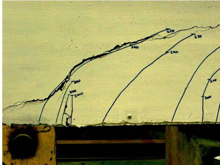
**Figure 5.22:** Left hand shear crack S4 B
