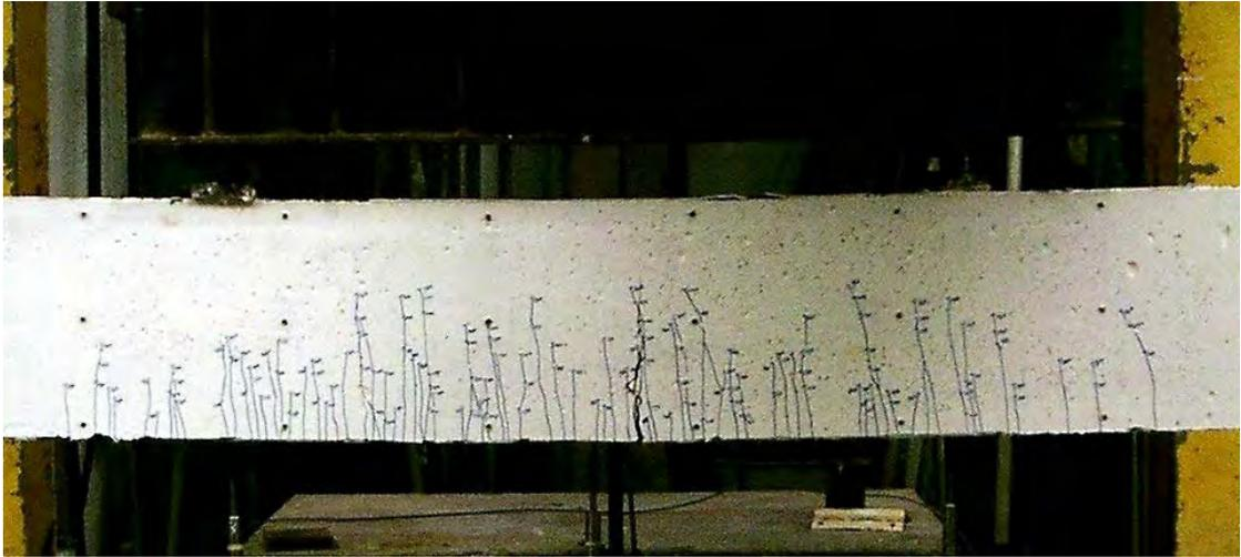
**Figure 5.18:** Final crack pattern in the constant moment region S2 A
