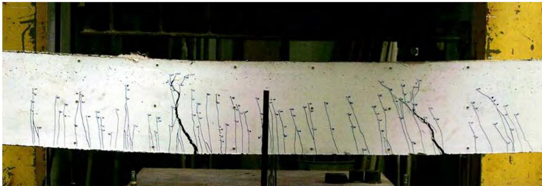
**Figure 5.17:** Final crack pattern in constant moment region S1 A
