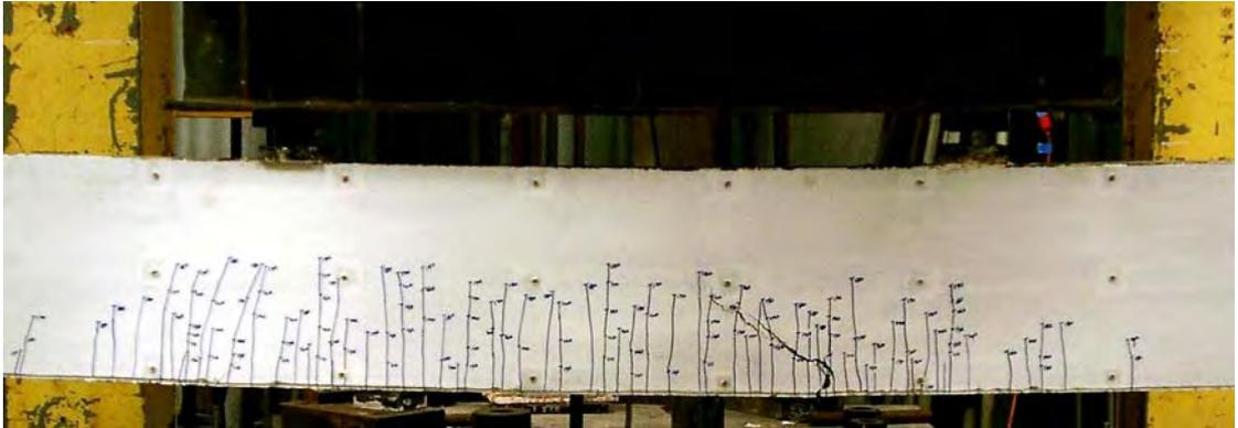
**Figure 5.20:** Final crack pattern in constant moment region S3 B
