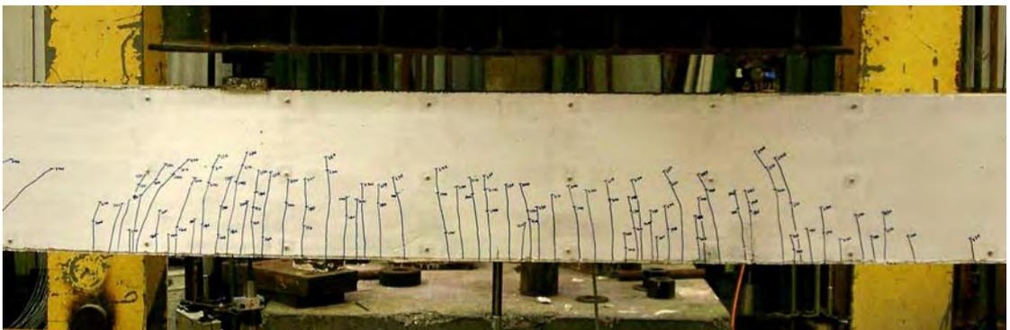
**Figure 5.21:** Final crack pattern in constant moment region S4 B
