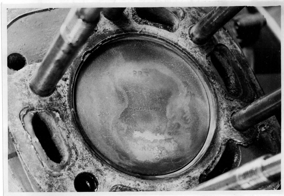
Fig. 42 - Carbon deposits on piston crown after the main tests.
