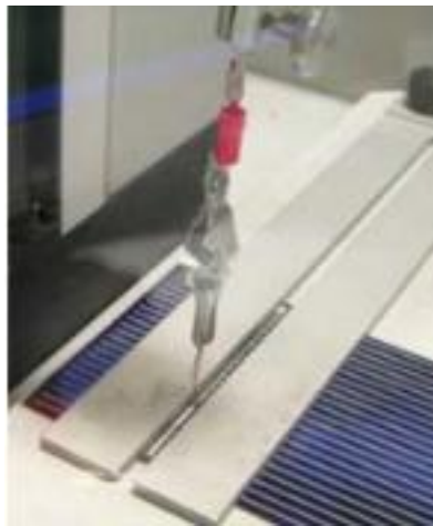
Figure 5-2. 90-degree pull test employed to reduce the chance of the solar cell breaking during measurement (from [333]).
