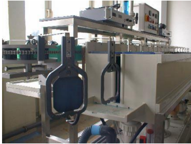
Figure 2-11. Photo of the electroplating arrangement trialled by BP Solar for their plating of LBG solar cells (from [124]).
