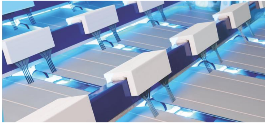
Figure 2-18. The Rena bias-assisted LIP tool InCellPlate with a brush contact at the rear and single side plating with wafer transport achieved by conveyer rollers (from [149]).
