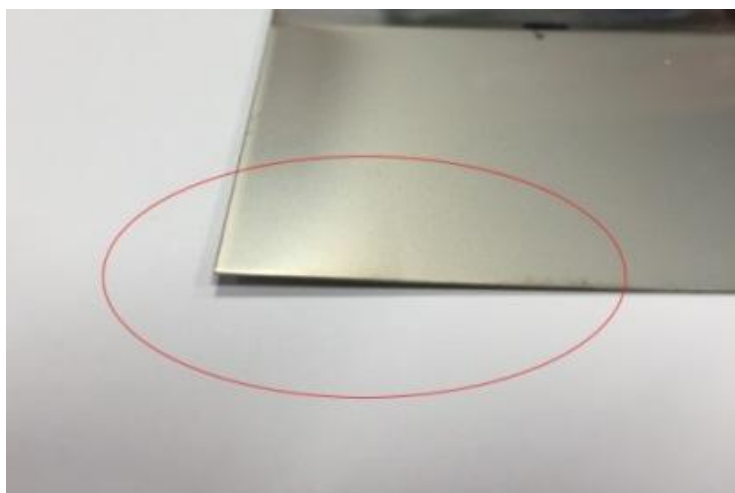
Figure 5-25. Plated Ni layer bending the flat cathode sheet in a Hull cell test due to use of a high plating current density.
