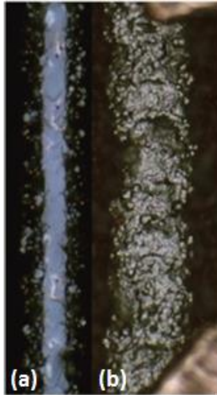
Figure 5-16. One-step Ni plating (i.e., Group A1) showing: (a) complete removal of the Ni layer for n-type laser-doped grooves; and (b) retention of the Ni layer after adhesion testing of a p-type laser-doped groove.
