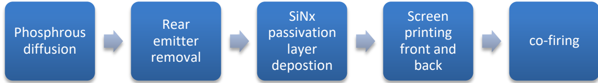
Figure 2-2. Process flow diagram for fabrication of a typical p-type Cz screen-printed Si solar cell.
