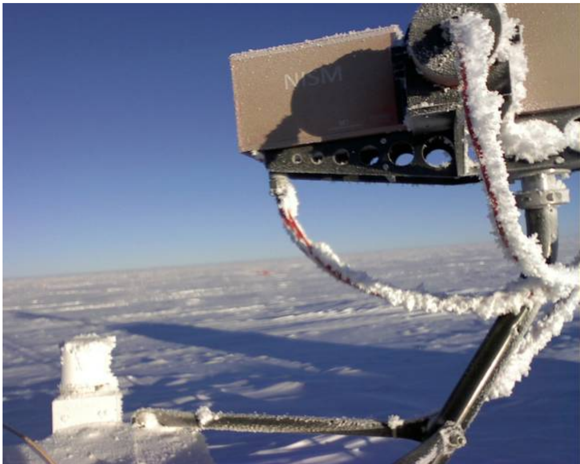
Figure 7.2: Ice on the back of NISM early in the season, on 2015-03-30 (From the Ridge A webcam).
