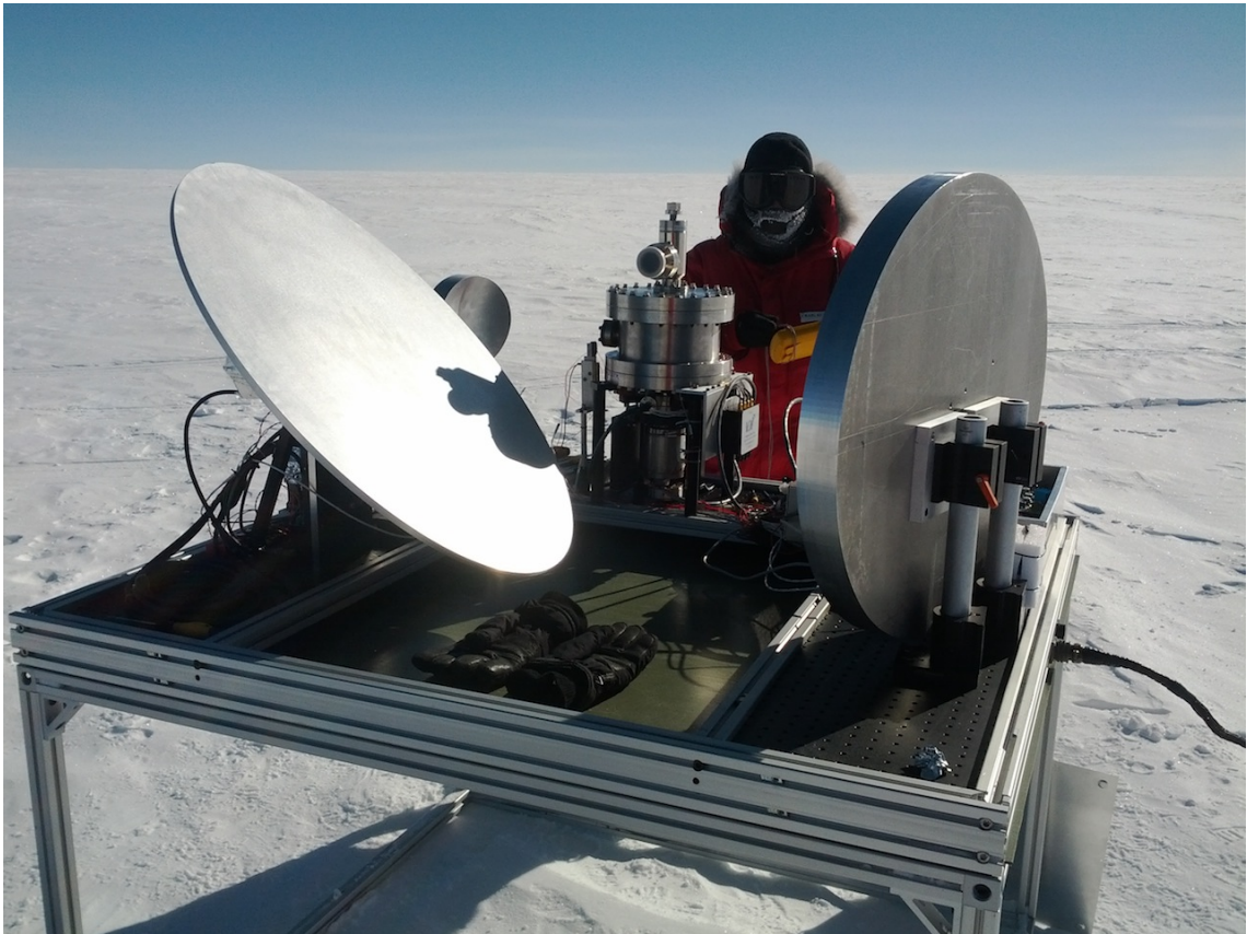
Figure 2.7: The HEAT telescope without its cover, showing the mirrors and cryostat. [Credit: Craig Kulesa, 2012]
