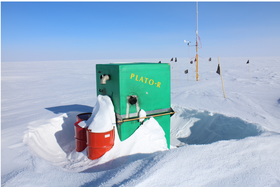
Figure 2.10: The PLATO-R Engine Module. The snow piles up and has to be dug away each season, resulting in the crater around the module.[Credit: Nic Bingham, 2015]
