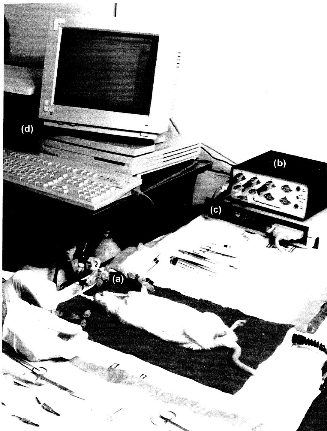
**Figure 8.2** Direct BP monitoring setup for PHF bioassay. (a) pressure transducer, (b) PA-100 amplifier, (c) Biopac MP-100, (d) Apple Macintosh running Acqknowledge data acquisition software.
