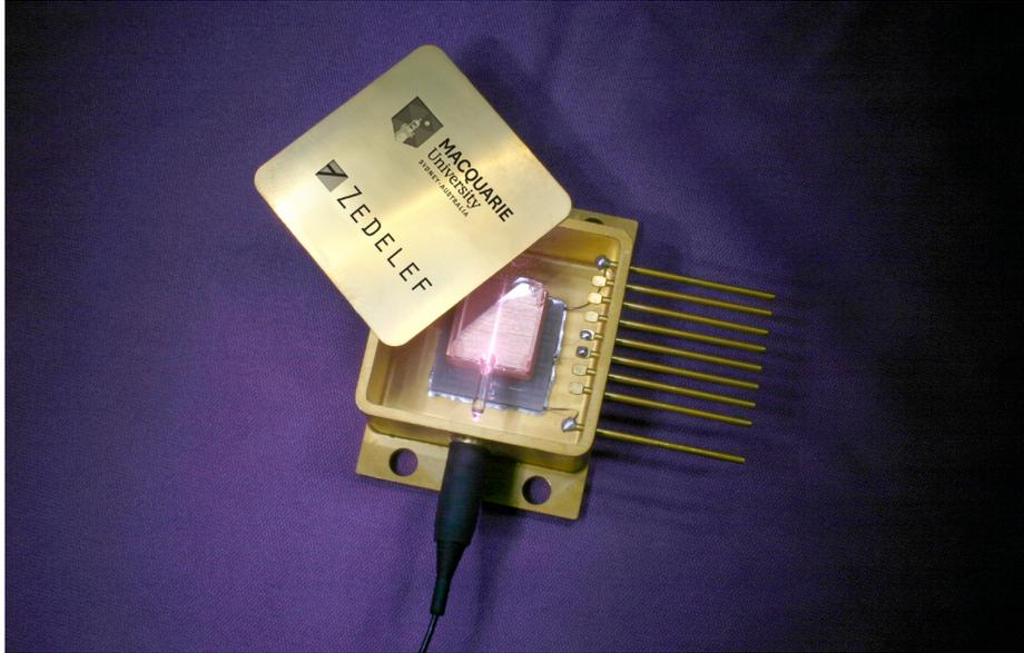
Fig. 1.9 Schematic of monolithic actively Q-switched waveguide lasers designed by the collaborators Zedelef Pty Ltd and Macquarie University.
