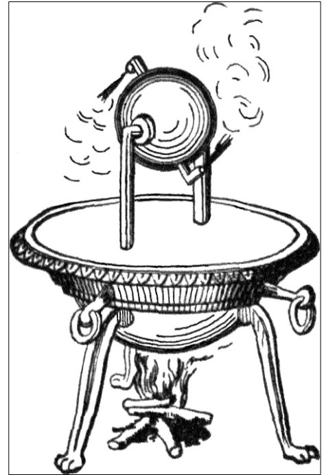
figure 1: Hero of Alexandria's Aeolipile.
