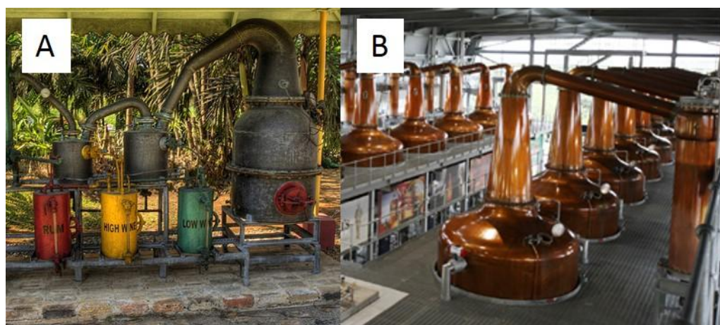
Figure 2.2 Pot stills used in the production of distilled spirit. (a) crude rum still (Artisan Distiller, 2011) (b) Scotch whisky production at Roseisle distillery, Scotland. (Sword 2010)
