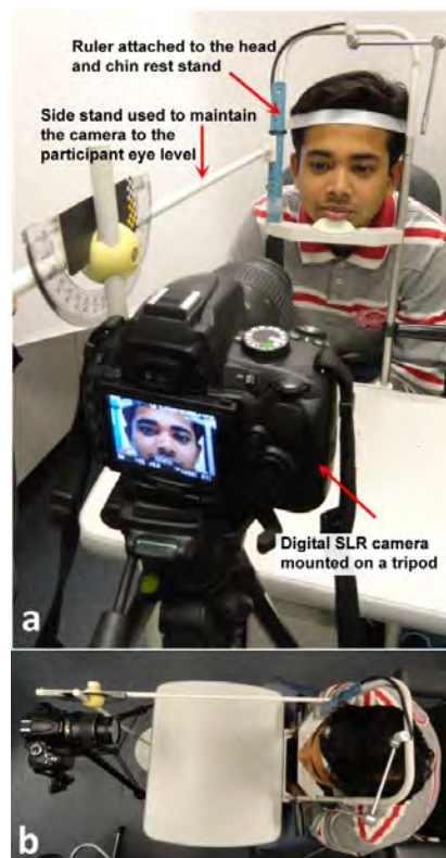
Figure 2-1. Set-up used for capturing eye photographs. a. view from behind the camera and b. view from above the camera and participant chin rest. Permission granted by participant for reproduction of this figure.
