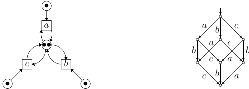
Fig. 10. A 2-out-of-3 semaphore , represented as a Petri net and as a higher dimensional automaton. In the latter, all six squares are supposed to be filled in, but the interior of the cube is not. Up to history preserving bisimulation equivalence this system cannot be represented as an automaton under the concurrent interpretation, because, due to the filled-in squares, the cube shape is unavoidable, and interior of the cube would by default be understood to be filled in. Hence the system can also not be represented as a pure Petri net.
