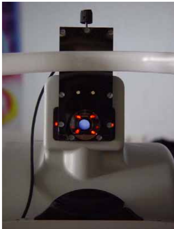
Figure 2.5: The off-axis target device attached to the measuring head of the COAS G200
