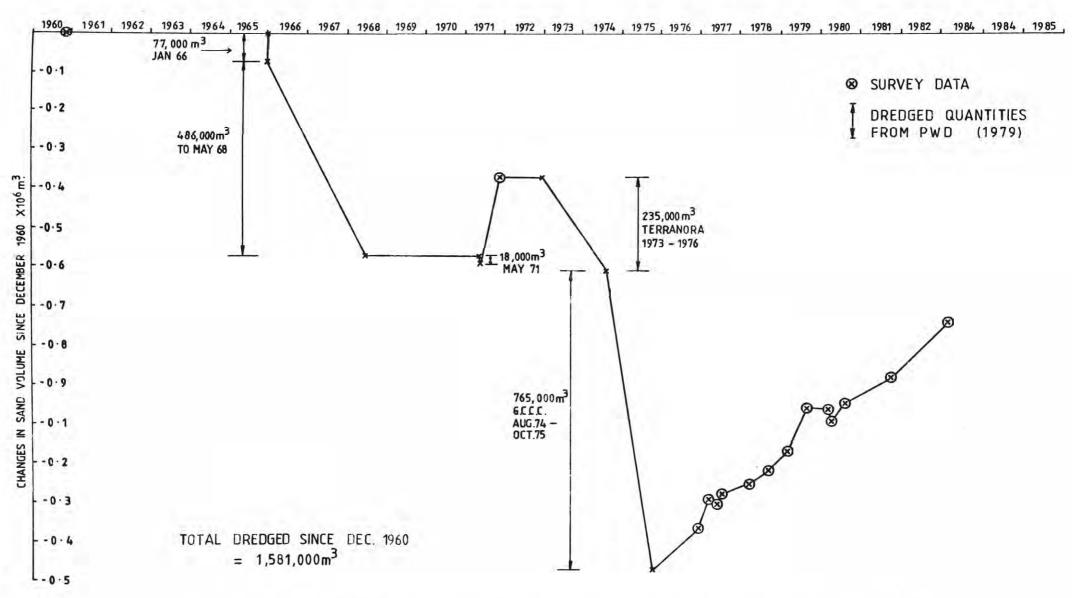
SCHEMATIC REPRESENTATION OF THE CHANGES IN THE TWEED RIVER CHANNEL CAPACITY DUE TO DREDGING AND SUBSEQUENT INFILLING
