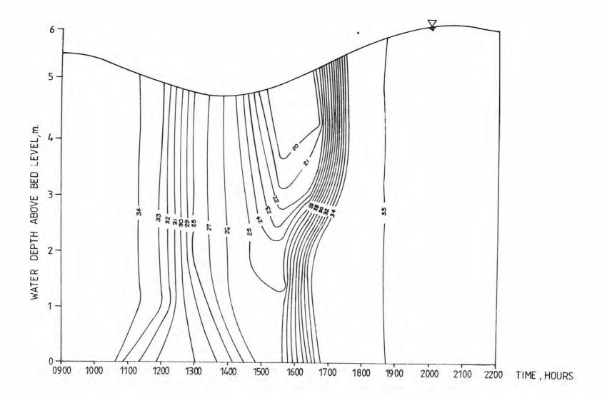
SALINITY DISTRIBUTION (IN PARTS PER THOUSAND) AT THE MID CHANNEL GAUGING STATION SHOWN ON FIGURE 10-20TH MAY 1985
