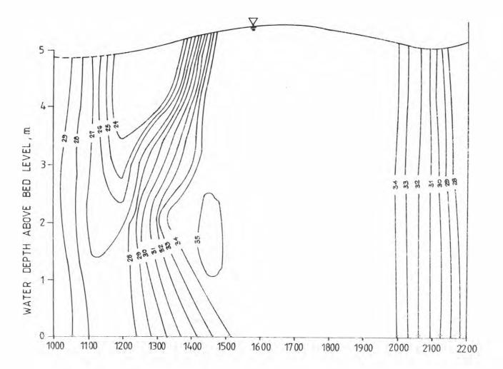
SALINITY DISTRIBUTION (IN PARTS PER THOUSAND) AT THE MID-CHANNEL GAUGING STATION SHOWN ON FIGURE 10-13TH MAY 1985
