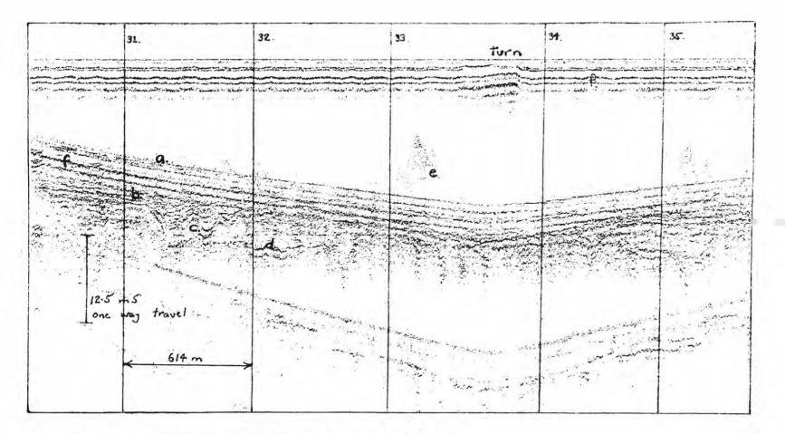
SEISMIC REPLAY RECORD. - KIRRA AREA. - FIXES 31-35.
