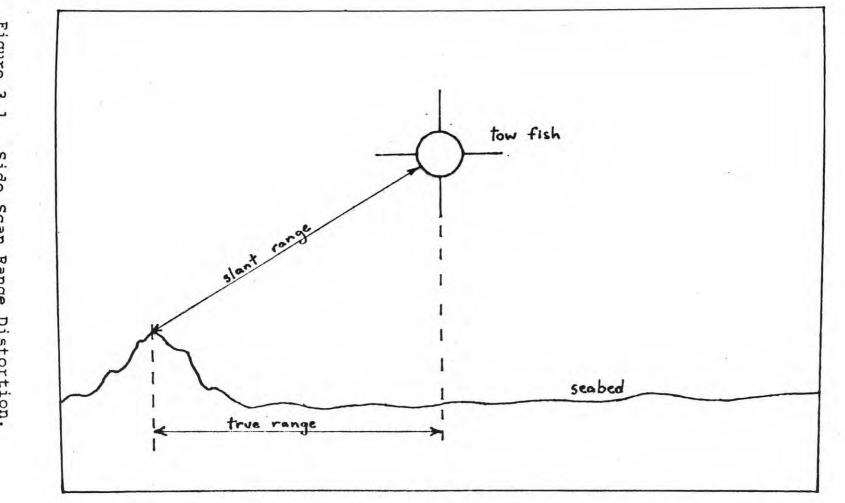
Figure 3.1. Side Scan Range Distortion.
