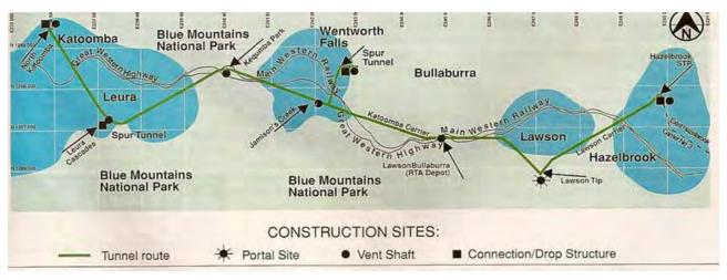
Figure 4.7: Positioning of the Blue Mountains Sewage Tunnel (Wallis 1995)
