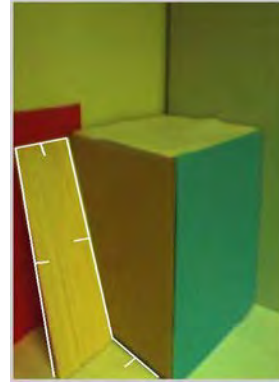
(b) Extracted image lines with falsely grouped line from wrong surface (ground).
