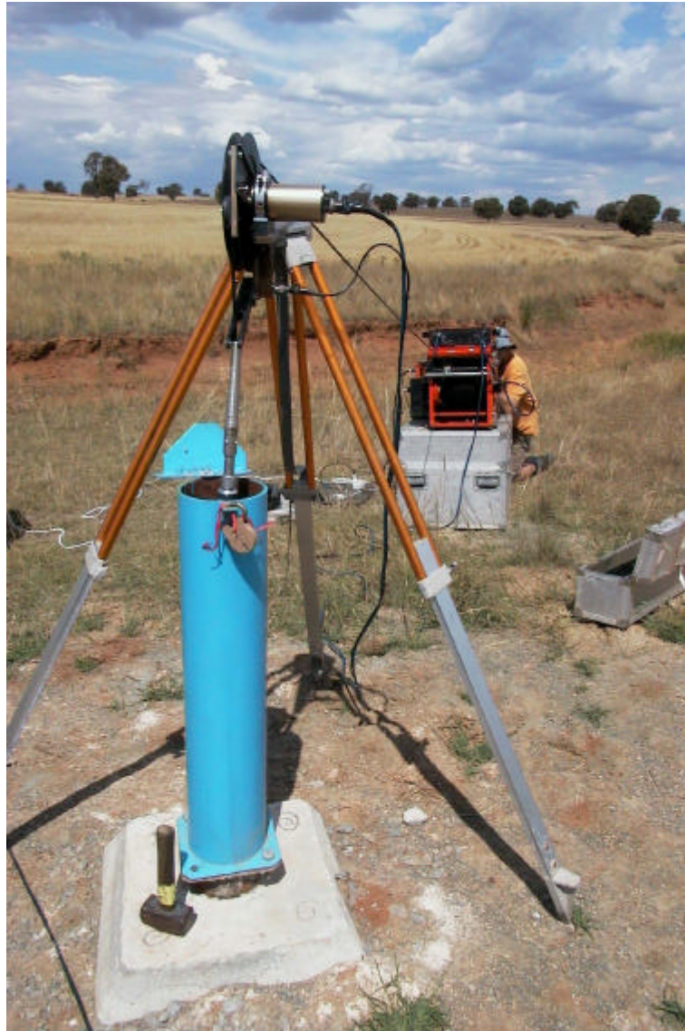
Figure 4.18: Borehole Geophysical Logging At GW96128 Site
