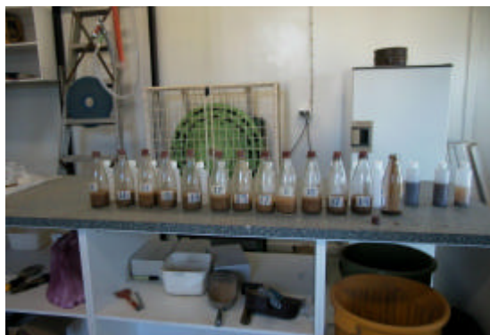
Figure 4.13: Aqueous 1:5 Extracts Settling Period Prior to Measurement
