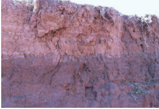
Figure 5.7: Salt Concentrating at the Top of the Capillary Zone in Unit One
