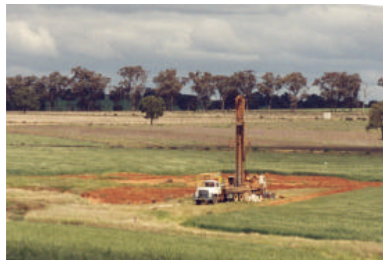
Figure 4.5: Drilling Nested Monitoring Bore Site GW96128
