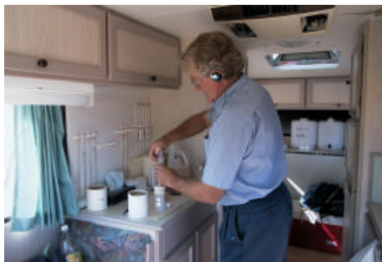
Figure 4.22: Filtering and Preservation of Water Samples
