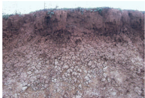
Figure 5.14: Hexagonal Shrinkage Cracks and Surface Frittering In Unit Two
