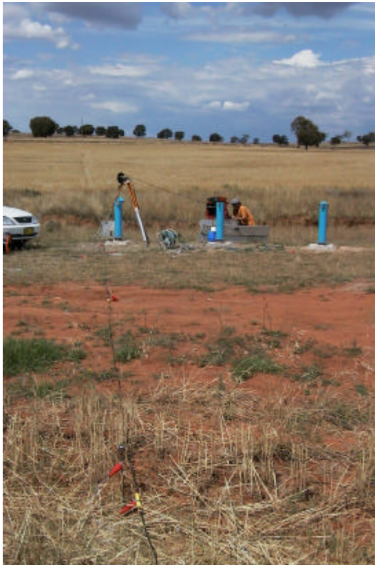
Figure 4.15: Electrical Resistivity Image Line One and Borehole Geophysical Logging at GW96128
