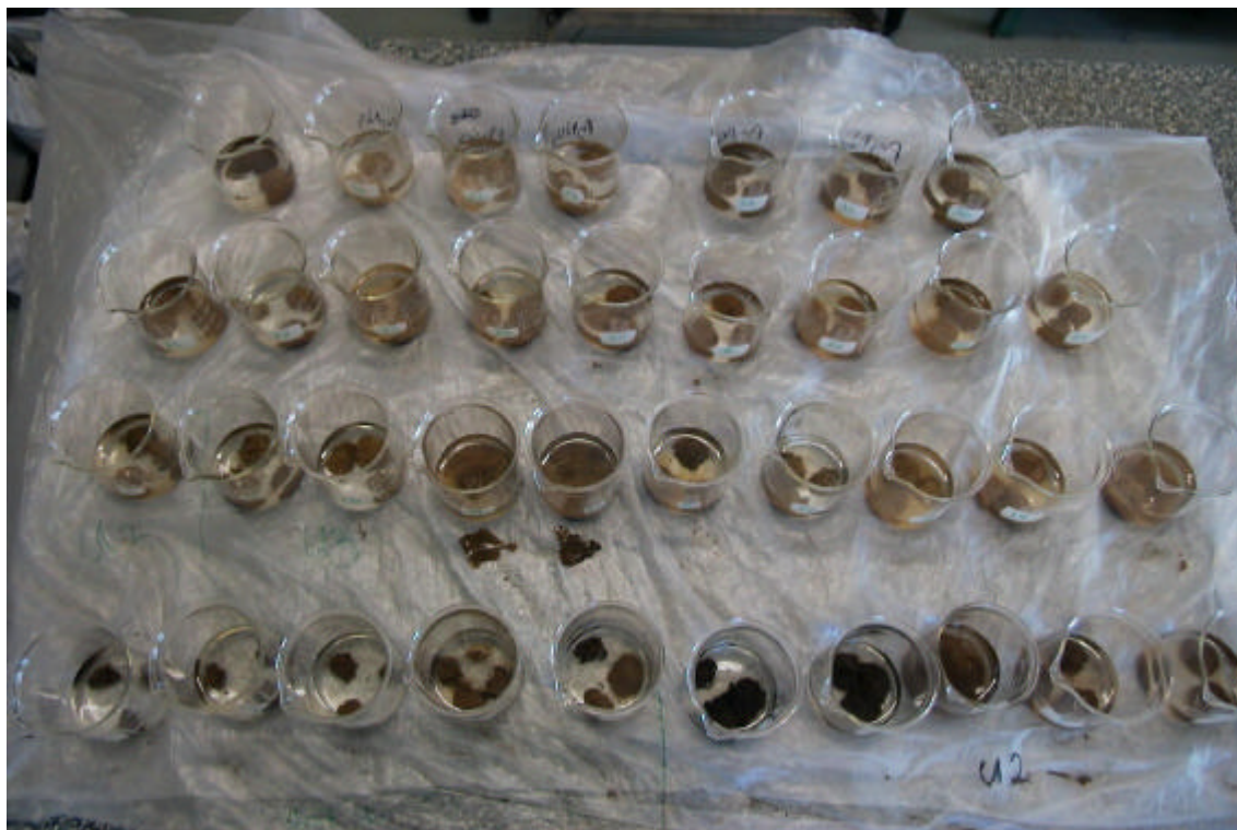
Figure 4.10: Emerson Aggregate Dispersion Testing
