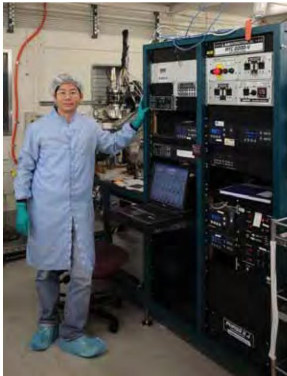
**Figure 1.3:** The ATC 2200 RF magnetron sputtering system, manufactured by AJA International, employed in this thesis.
