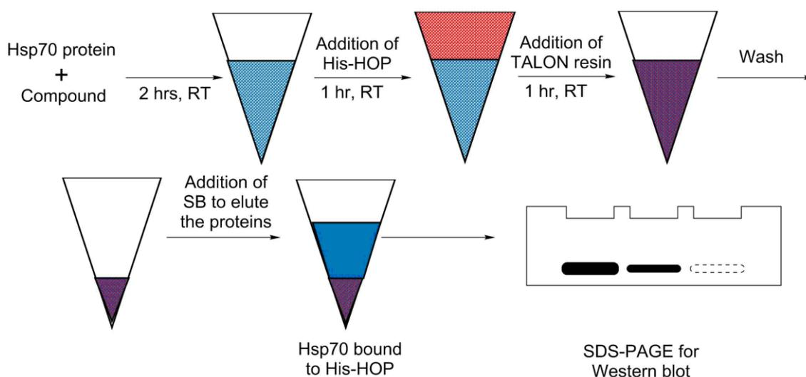
**Figure 2. 10** : Schematic for pulldown assay
