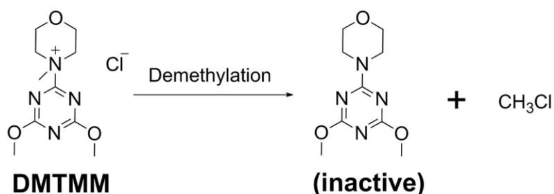
**Scheme 2. 4:** Decomposed of DMTMM to an inactive molecule.
