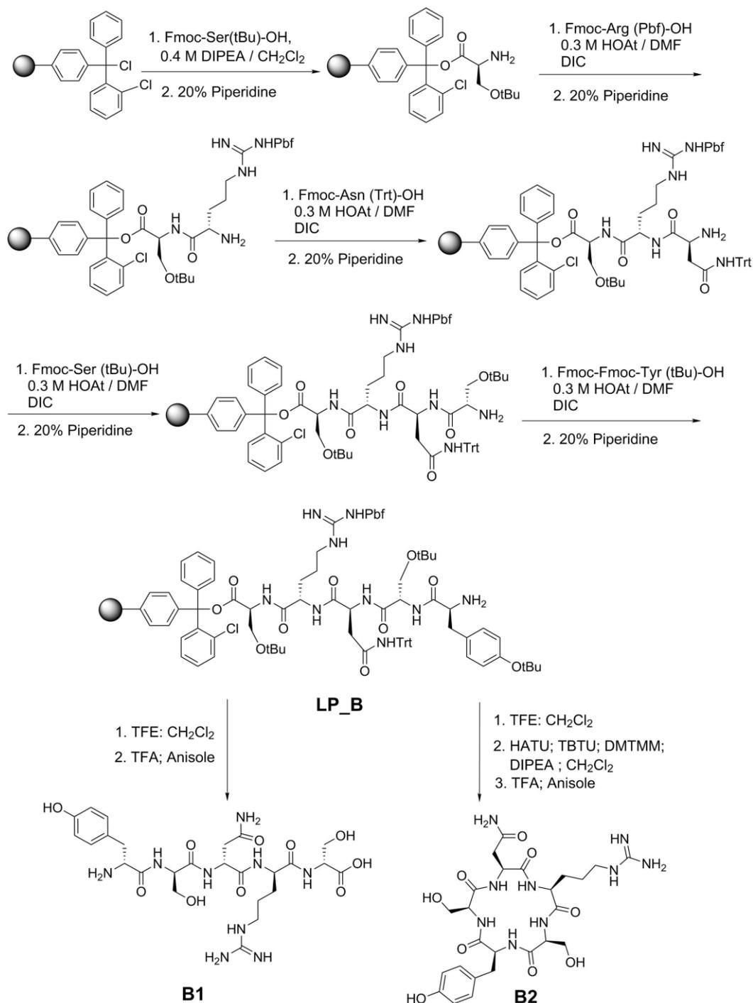
**Scheme 2. 2:** The synthesis scheme for **B1** and **B2**.
