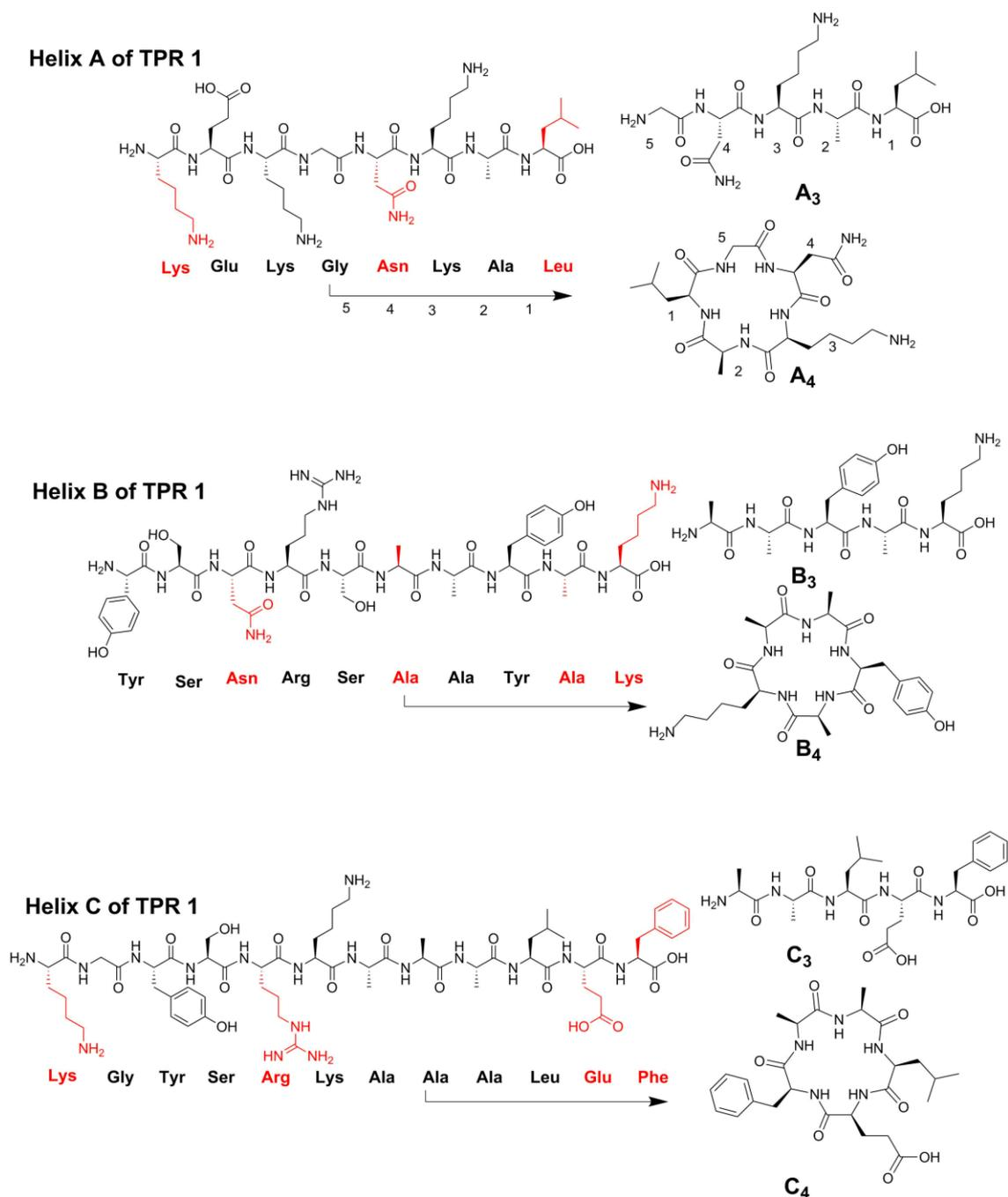
**Figure 2. 5:** Structure of analogues that were designed based on the C-terminus of helices A, B and C. Final structures produced were molecules A3, A4, B3, B4, C3 and C4.
