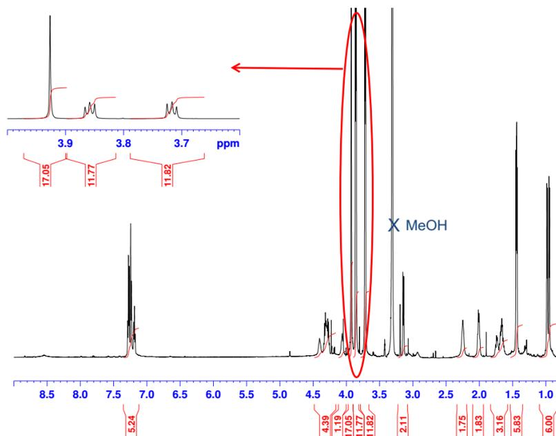
**Figure 2. 7:** Structure and <sup>1</sup>H NMR spectrum of **C4**. The highlight peaks belong to impurity
