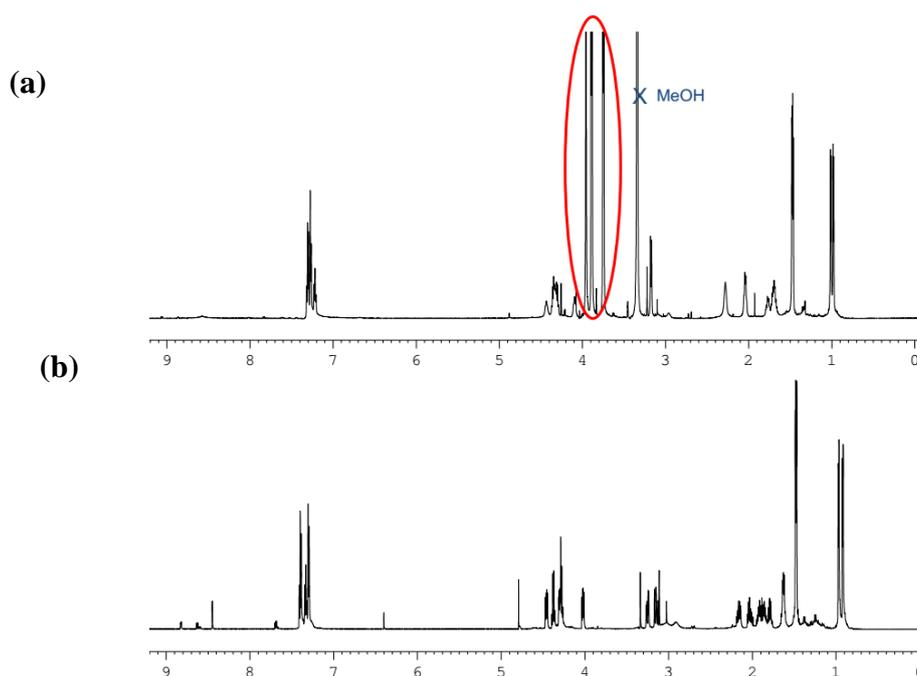
**Figure 2. 9:**  $^1\text{H}$  NMR spectrum of **C4**. a) The highlighted peaks belong to impurity when the compound was first synthesized. b) spectrum belongs to **C4** when the compound was synthesized without DMTMM. This spectrum lacks impurity peaks.
