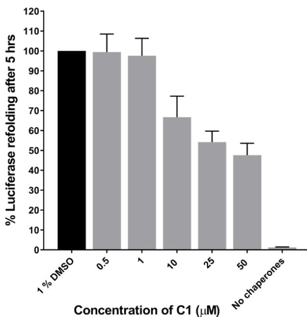
**Figure 2. 18:** The impact of C1 at multiple concentrations on luciferase refolding after 5 hours. The graphs represent the mean  $\pm$  SEM, from at least three independent experiments.
