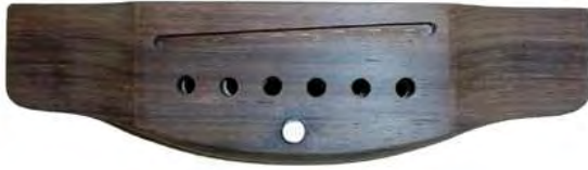
Figure E.3: One of the guitar bridges with an embedded rare-earth magnet to couple the instrument to the excitation/detection apparatus. The visual effect is not unæsthetic
