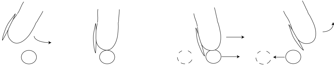
Figure 2.6: The action of plucking a guitar string. Shown are the relative positions of the finger-tip and the string, as viewed along the string axis, before, during and after the plucking action. The arrows represent the relative velocities, the dotted circles are the initial positions of the string.
