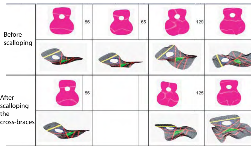
Figure 4.11: Calculation of normal modes of a free soundboard of a steel-string acoustic guitar with standard Martin cross-bracing, after scalping the cross-braces only. From [Vernet, 2001].
