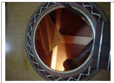
Figure 3.13: Photograph of the set-up for the scalloping procedure after the soundboard has been attached to the back and sides.
