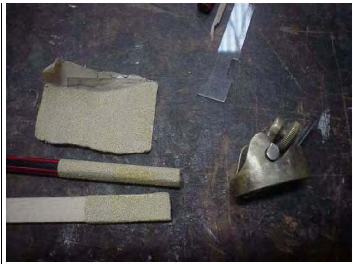
Figure 3.12: The tools used in scalloping the tone-braces.
