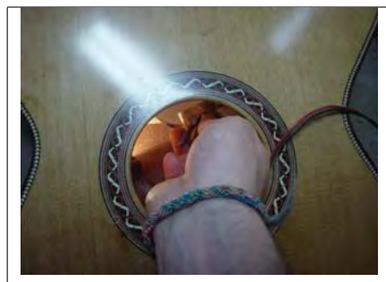
Figure 3.14: A luthier scallops the braces with a small thumb-plane, working from inside the sound-hole.
