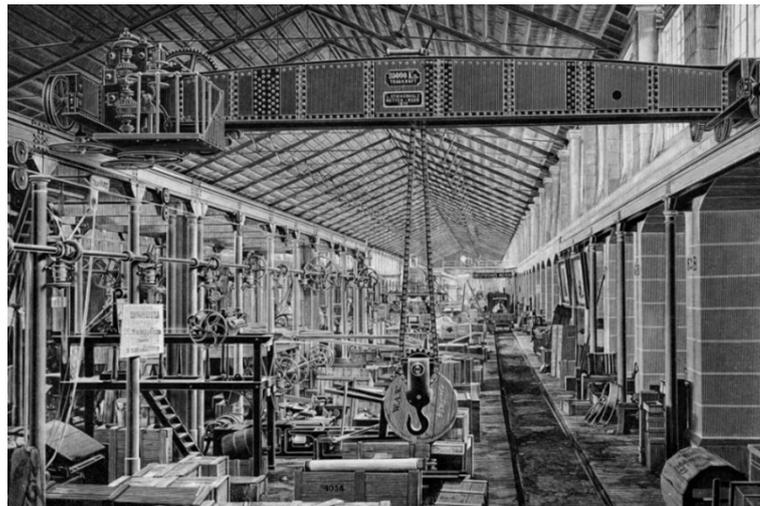
Fig. 4.1–1. A steam-powered overhead crane produced by Stuckenholz AG, Germany in 1875 [100].
