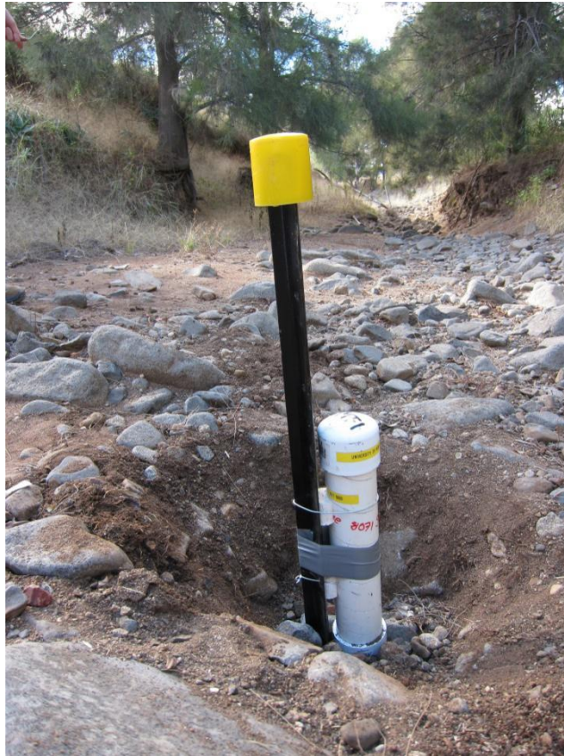
Figure 2.3 Monitoring stream level at a site similar to Middle Creek Farm.
