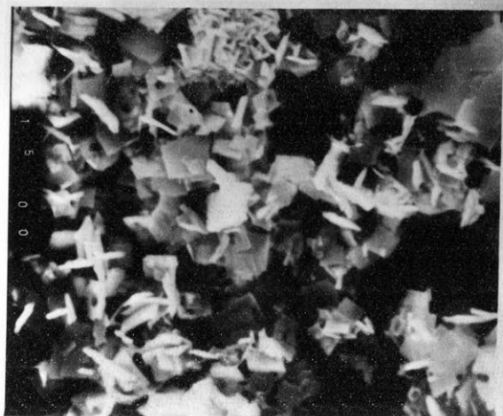
Figure 8.15. Scanning Electron Micrographs of Thorium Oxide Derived from the Oxalate Precipitated at 70 C
