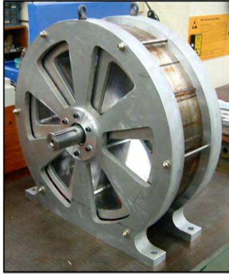
Fig.B. 7. FSCW IPMM-F machine assembly
