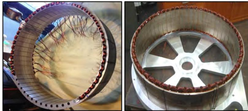
Fig.B. 6. Complete winding of the stator
