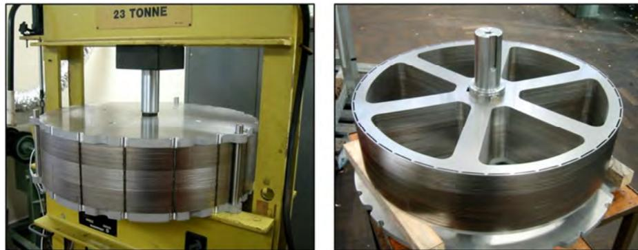
Fig.B. 4. Stacking of all rotor laminations
