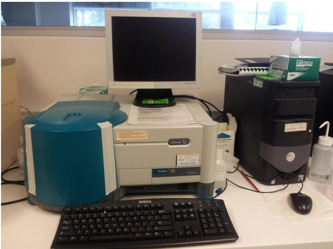
Figure 3.4 Fluorescence spectrophotometer
