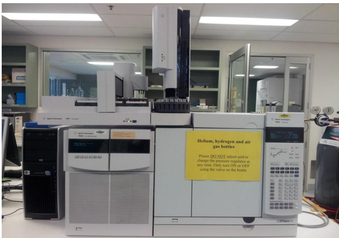
Figure 3.3 Gas chromatography tandem mass spectrometry
