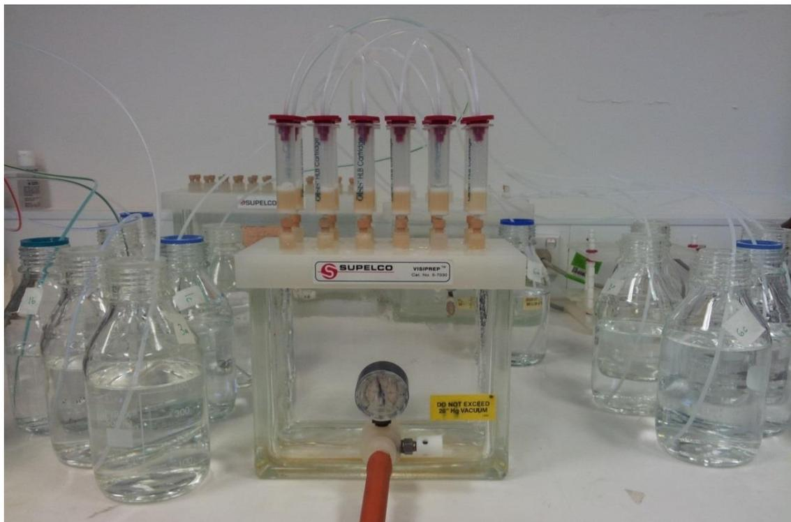
Figure 3.1 Solid phase extraction
