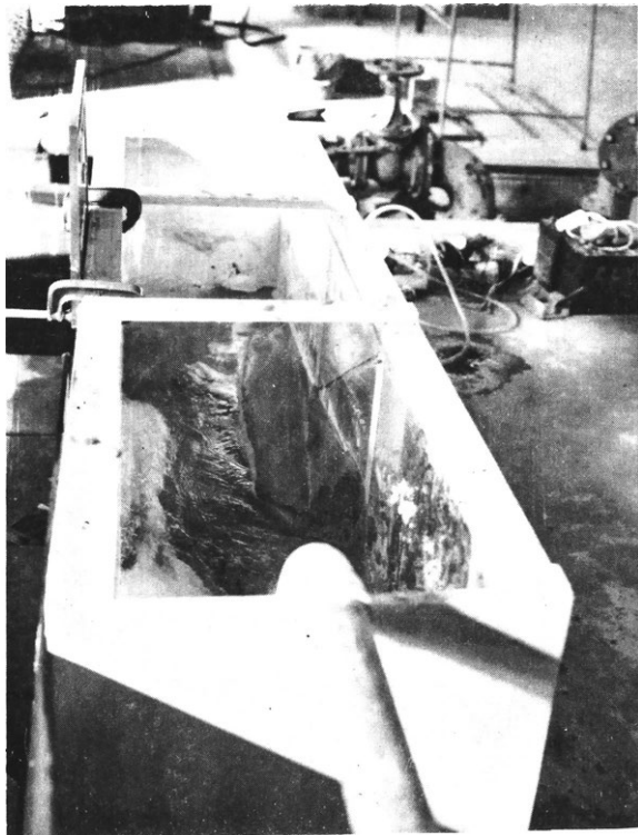
Fig.2: Hanging up of sand on side walls during flushing period. (No baffle).
