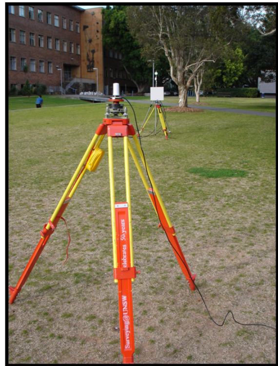
Figure 4. Left: 17mm Plexiglas obstructing antenna 5. Right: Rover antenna tracking LocataLite, with antenna 2 obstructed by 10mm plasterboard in the background.
