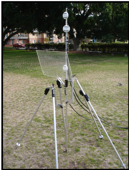
Figure 4. Left: 17mm Plexiglas obstructing antenna 5. Right: Rover antenna tracking LocataLite, with antenna 2 obstructed by 10mm plasterboard in the background.
