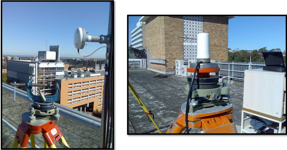
Figure 2. Left: A double clasp on a tripod, used to hold up materials in front of the transmitting antenna of the LocataLite. Right: The rover antenna connected to a laptop to record Locata signals at 2.4 GHz
