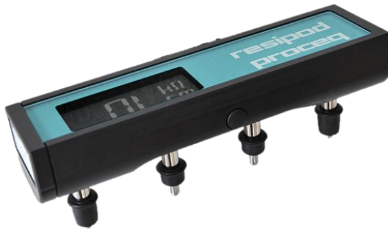
Figure 3.1 - Proceq Resipod four-point Wenner probe array
