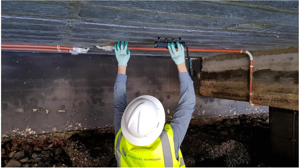
Figure 5.6 – Onsite resistivity testing using Proceq Resipod
