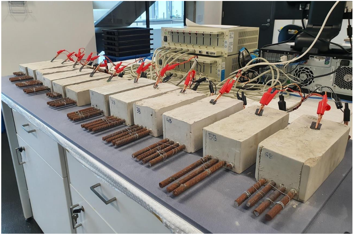
Figure 4.13 - Experiment 6 - resistivity measurement concrete sample
