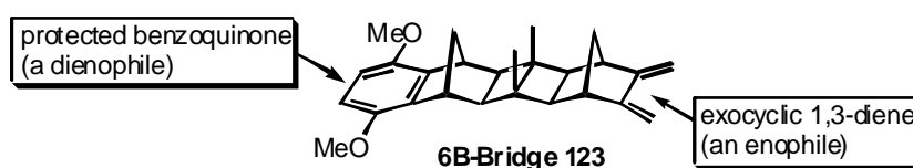
Figure 61: Norbornylogous bridge designed for the attachment of donor and acceptor moieties via Diels-Alder methodology
